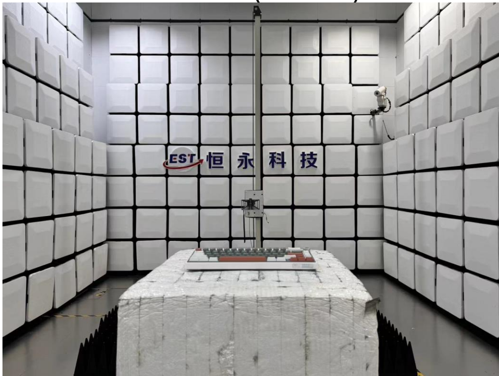
Radiated Test (Above 1GHz)
