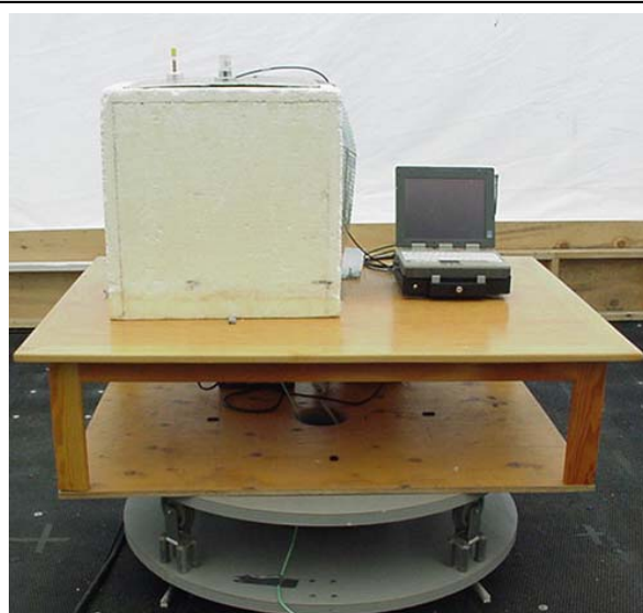
Photograph C.7-6 - Back of Radiated Emissions Setup with vehicle-mount antenna and cradle
