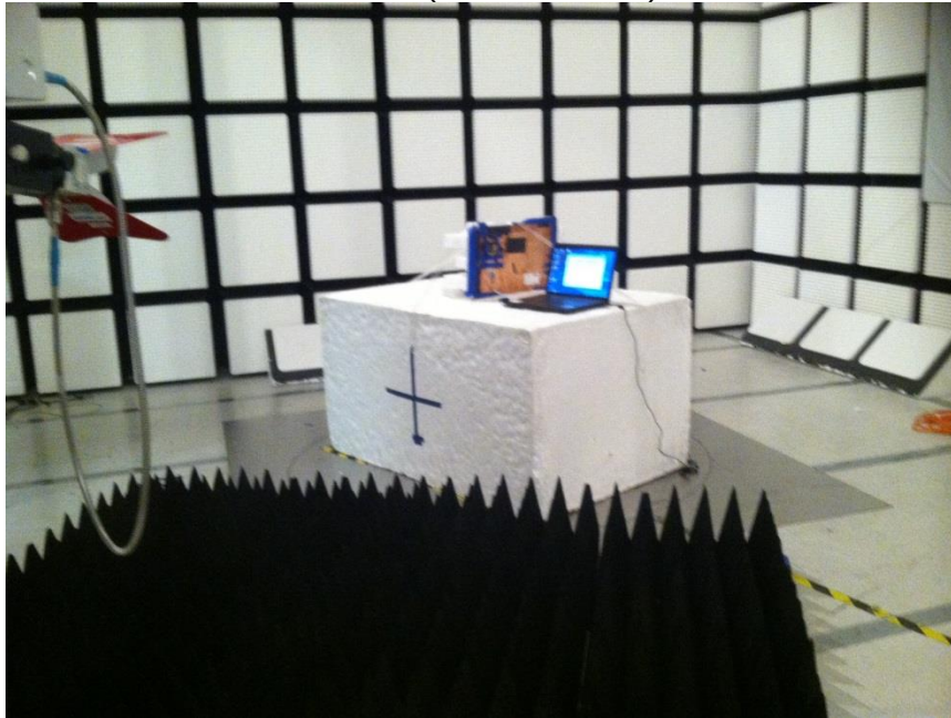
RADIATED FRONT PHOTO (ABOVE 1 GHz)
