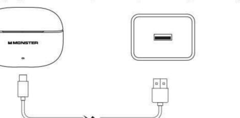
Rated input: 5V === 40mA(Headphone) Rated input: 5V === 200mA (charging case)
