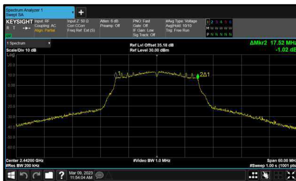
Figure 69 - 802.11n HT20 Minimum 99% OBW
