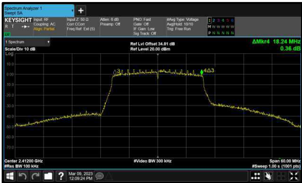
Figure 63 - 802.11ax HE20 SU Minimum 6 dB EBW
