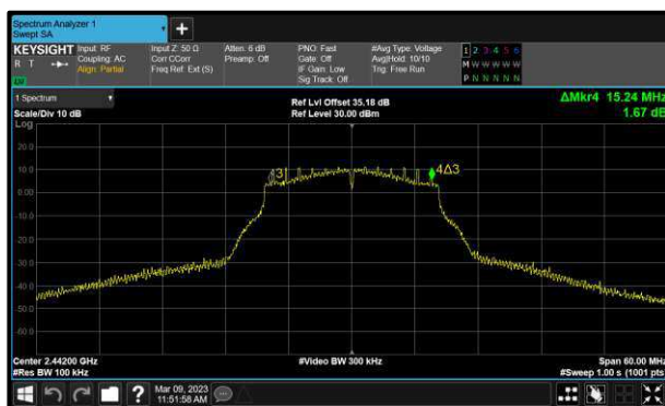
Figure 55 - 802.11g Minimum 6 dB EBW
