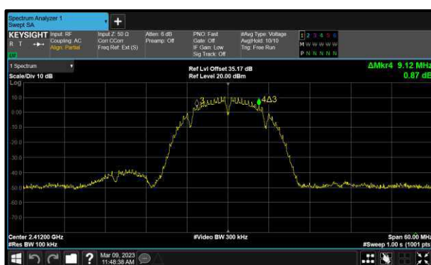
Figure 53 - 802.11b Minimum 6 dB EBW
