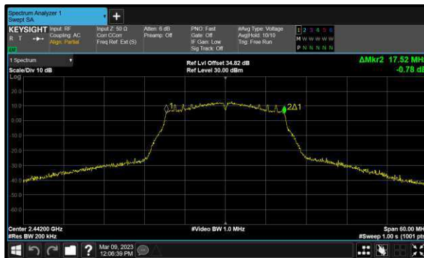
Figure 73 - 802.11n HT20 Minimum 99% OBW
