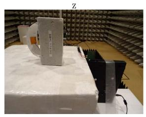
The antenna was tested with attached to supporting jig that does not affect EMC characteristic in order to place for each axis.
