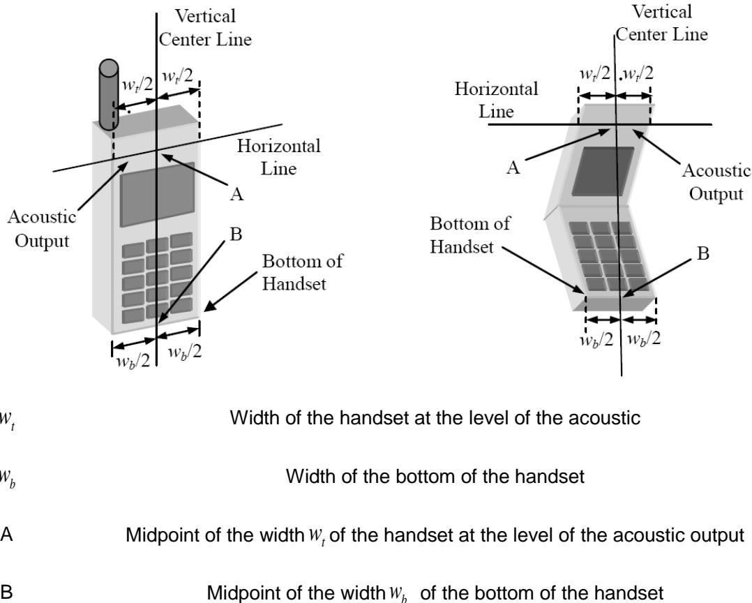
**Picture D.1-a Typical “fixed” case handset      Picture D.1-b Typical “clam-shell” case handset**
