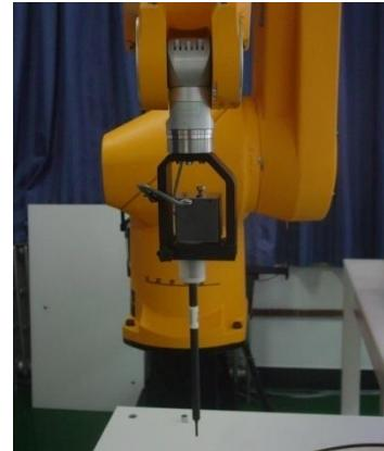
Picture C.3 E-field Probe
