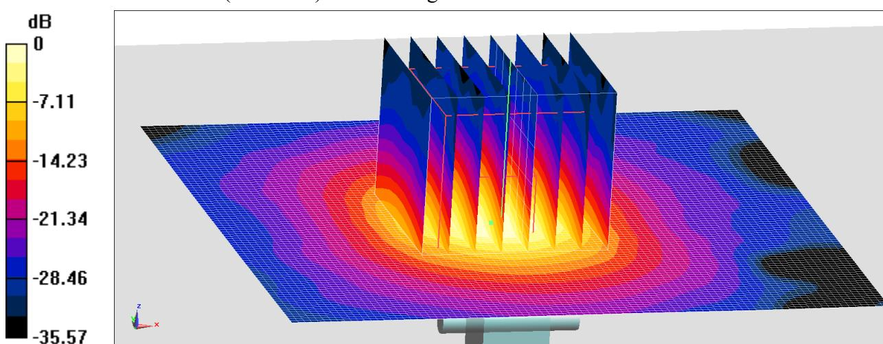
**Fig.B.8 validation 5750 MHz 100mW**
