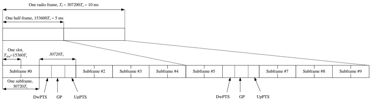
**Figure 9.2: Frame structure type 2 (for 5 ms switch-point periodicity)**
