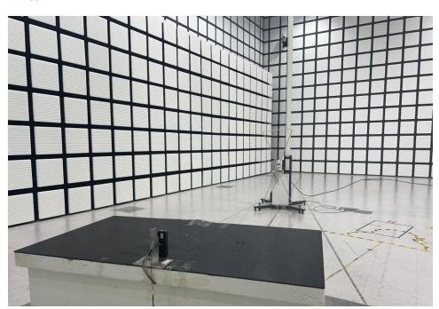
3. Radiated Emission setup photo (Above 1 GHz~18 GHz)
