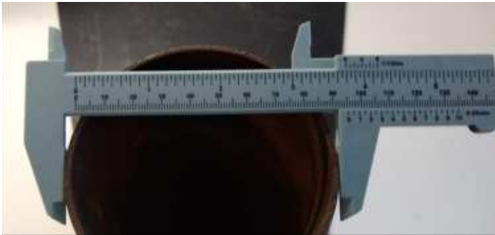
Figure 3: Measure Pole Diameter
