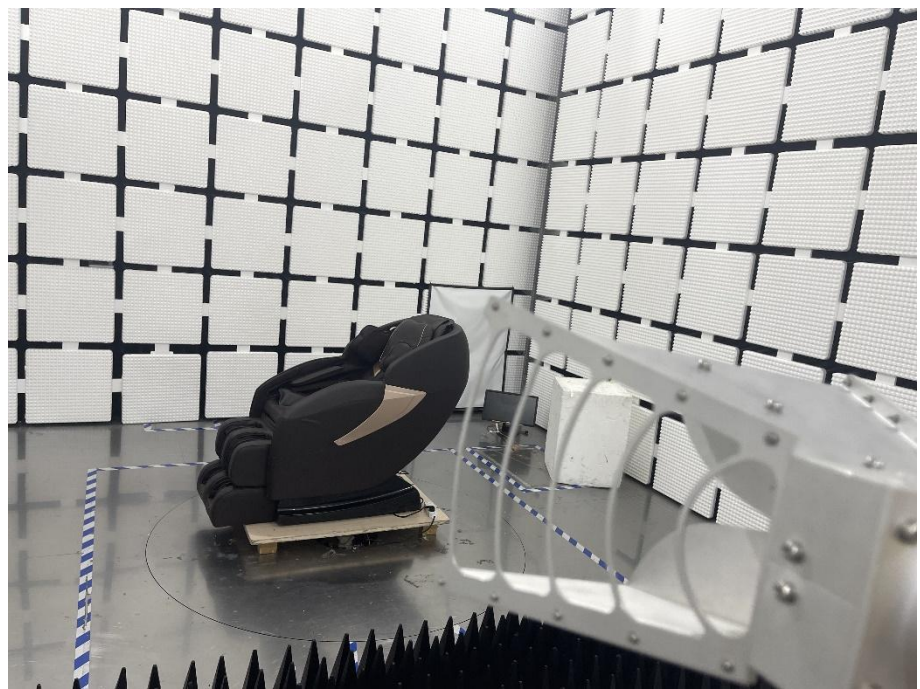
Radiation Emission Test Setup (1GHz to 18GHz)
