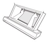
4 Hold the top of the auto-lift device with both hands and remove it from the bottom drawer.
