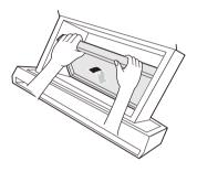
7 Lower the device into place and move it back and forth to make sure it is engaged.
