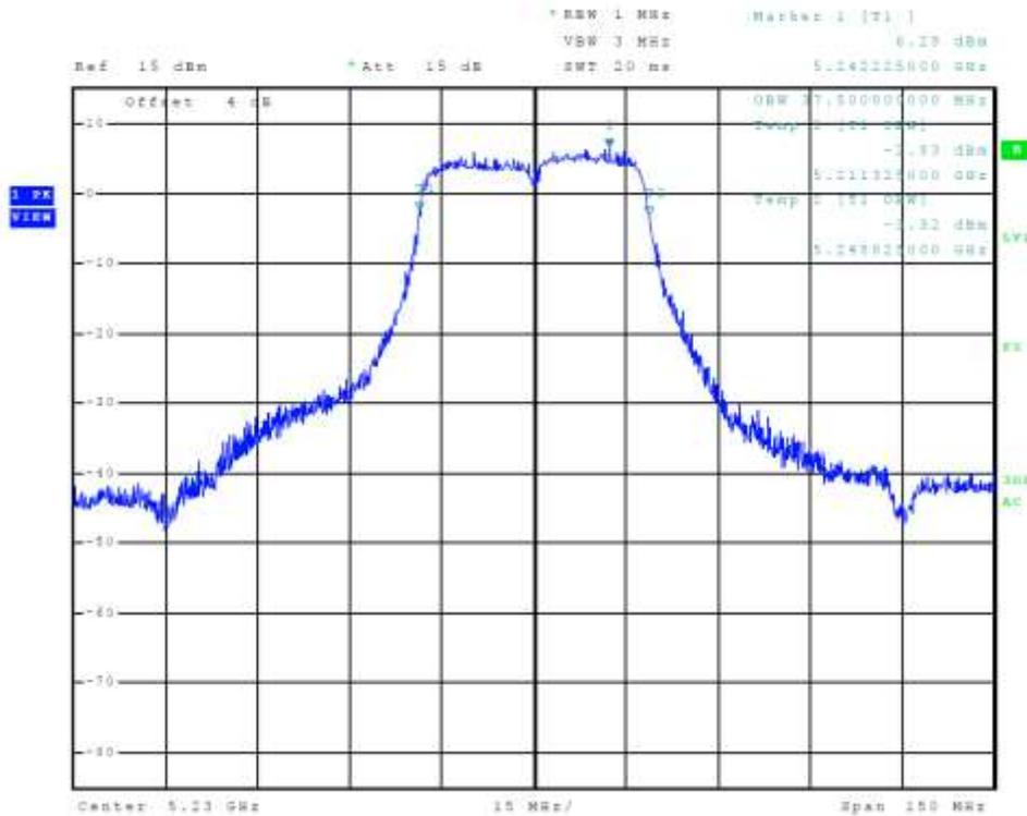
Figure 31 Plot of Transmitter Emissions Chain 1 (5150-5250 MHz Band, 802.11n40, 99% OBW)
