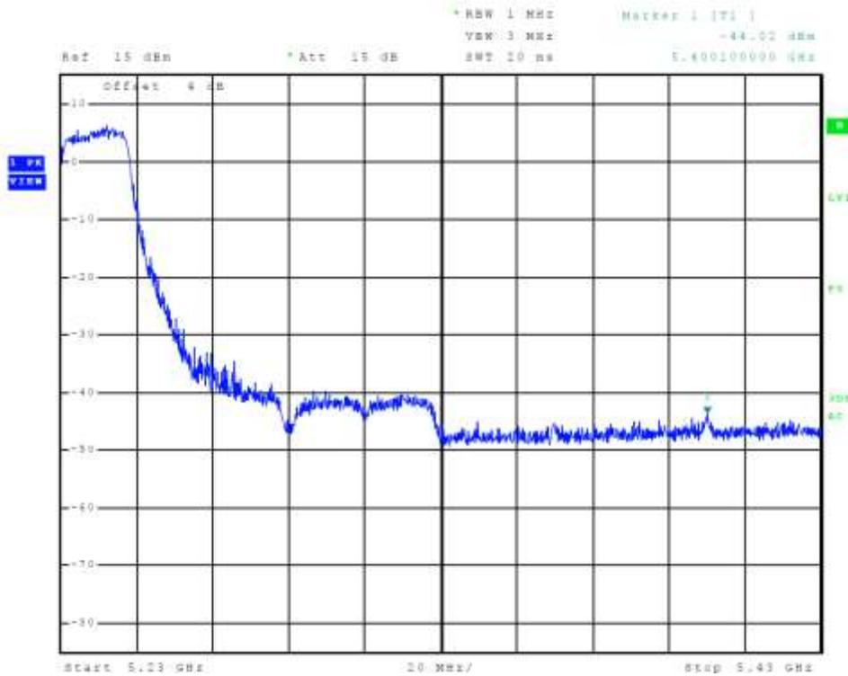
Figure 28 Plot of Transmitter High Band Edge Chain 1 (5150-5250 MHz Band, 802.11n40)
