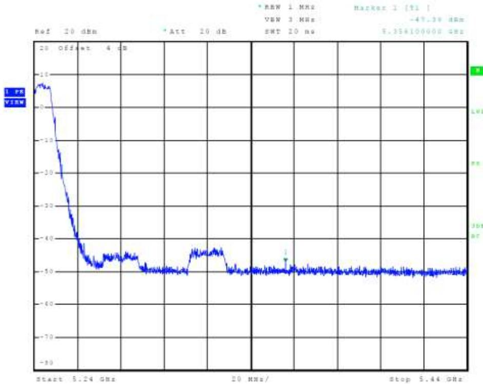
**Figure 7 Plot of Transmitter High Band Edge Chain 0 (5150-5250 MHz Band, 802.11a)**
