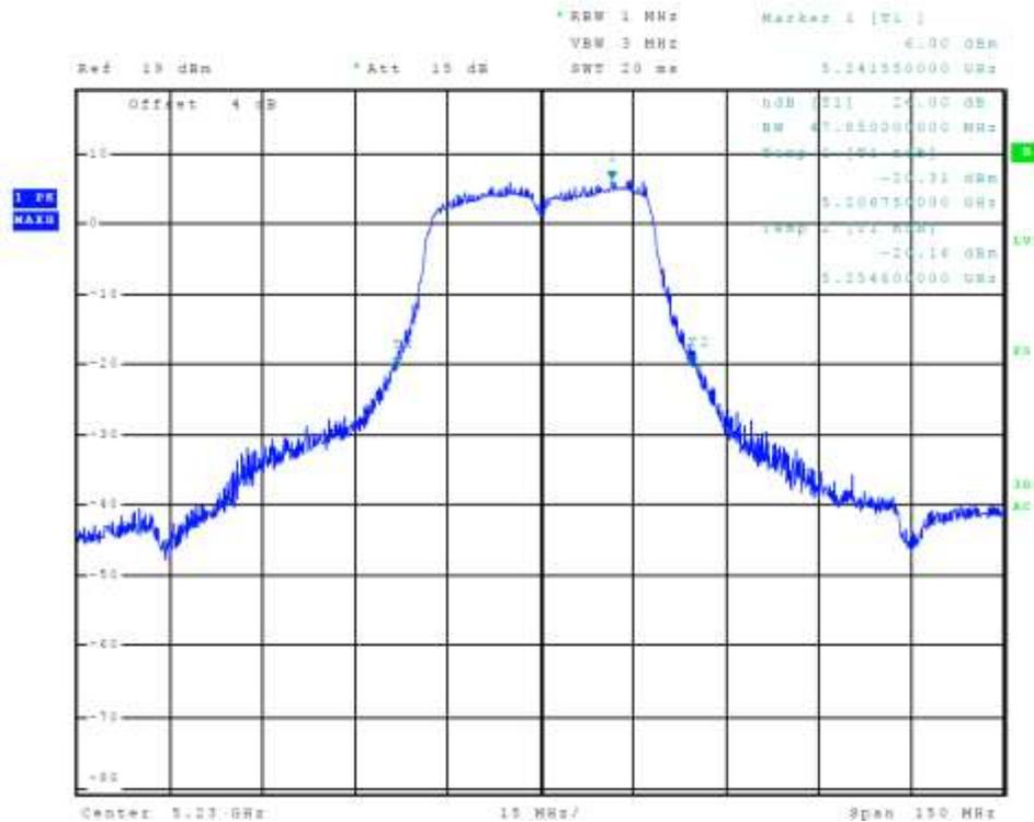
Figure 32 Plot of Transmitter Emissions Chain 1 (5150-5250 MHz Band, 802.11n40, 26 dB OBW)
