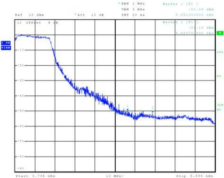
Figure 18 Plot of Transmitter High Band Edge Chain 0 (5725-5850 MHz Band, 802.11n40)
