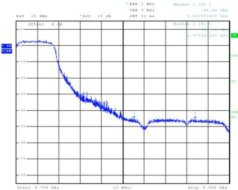
Figure 38 Plot of Transmitter High Band Edge Chain 1 (5725-5850 MHz Band, 802.11n40)
