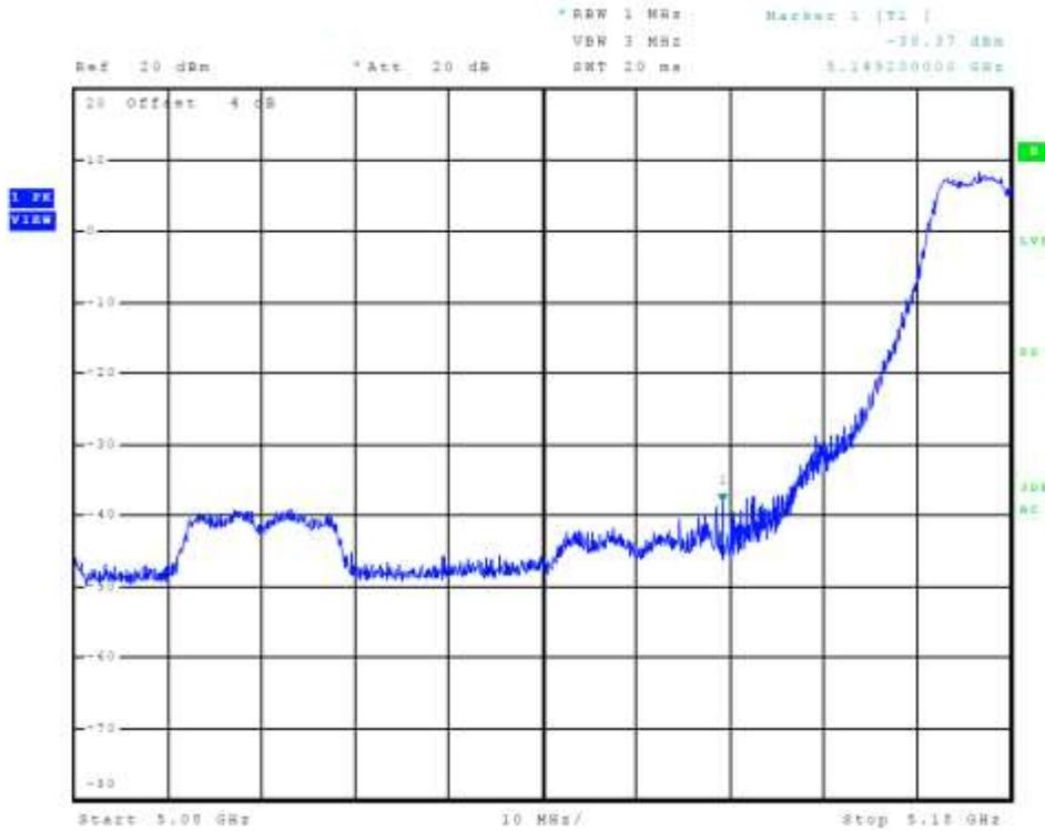
Figure 5 Plot of Transmitter Low Band Edge Chain 0 (5150-5250 MHz Band, 802.11a)
