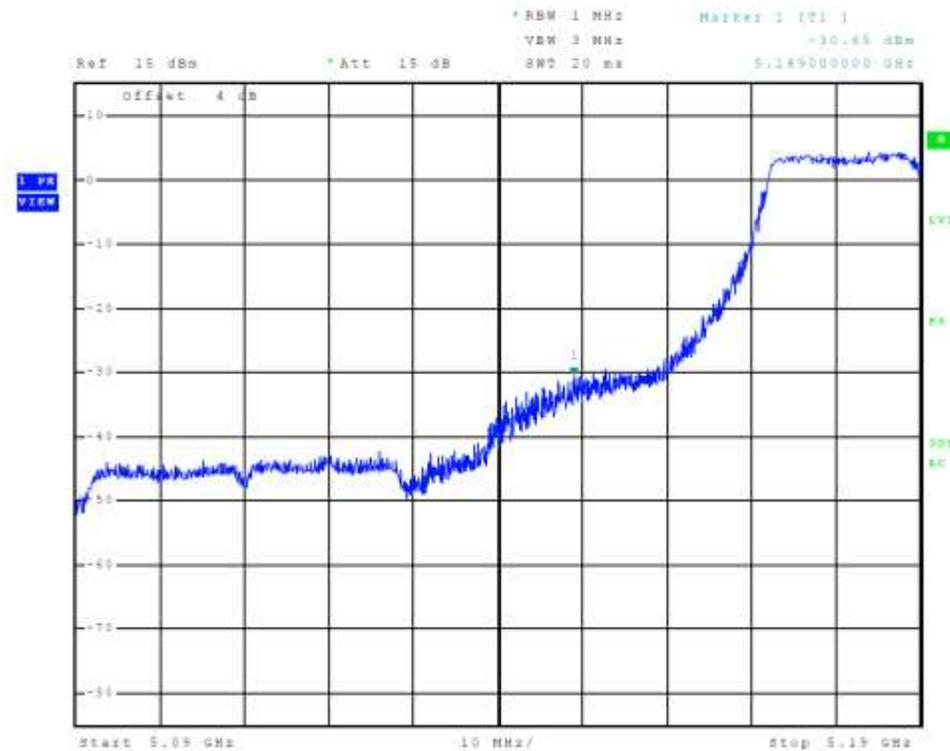
Figure 6 Plot of Transmitter Low Band Edge Chain 0 (5150-5250 MHz Band, 802.11n40)
