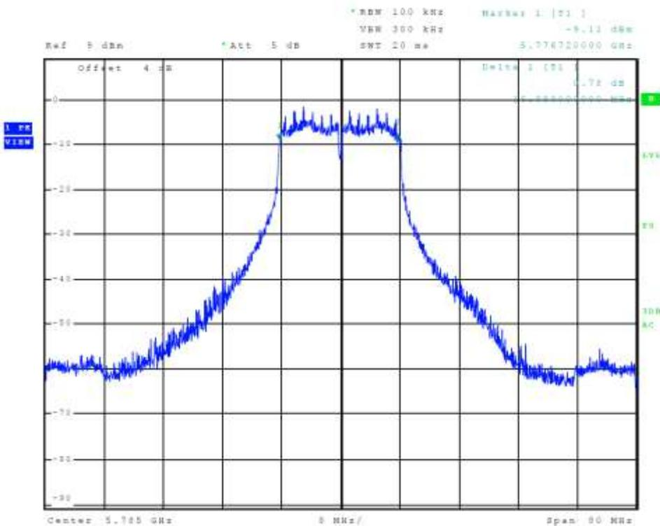
Figure 20 Plot of Transmitter Emissions Chain 0 (5725-5850 MHz Band, 802.11a, 6-dB OBW)
