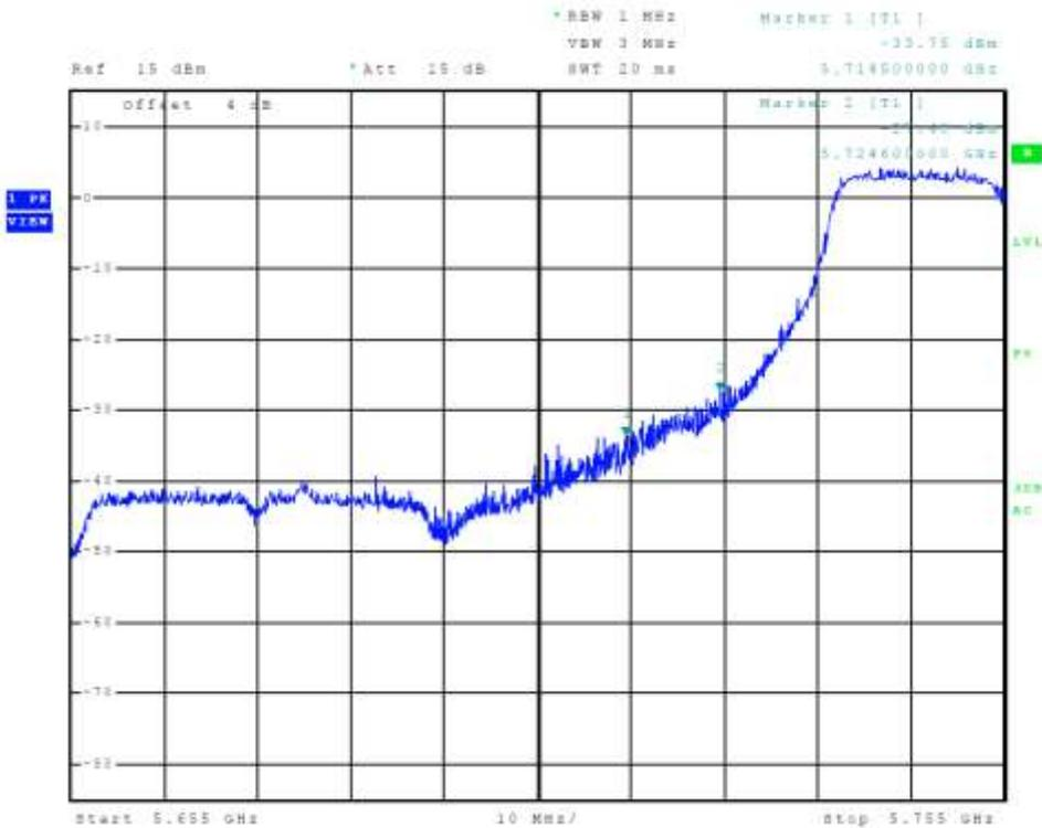
Figure 36 Plot of Transmitter Low Band Edge Chain 1 (5725-5850 MHz Band, 802.11n40)
