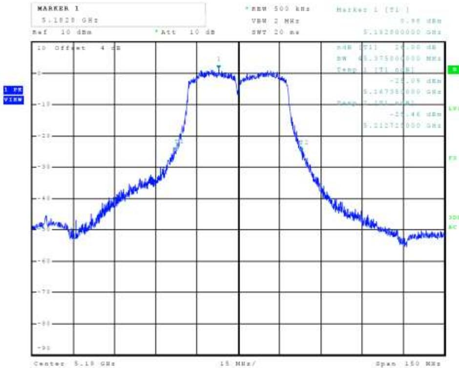
Figure 12 Plot of Transmitter Emissions Chain 0 (5150-5250 MHz Band, 802.11n40, 26 dB OBW)
