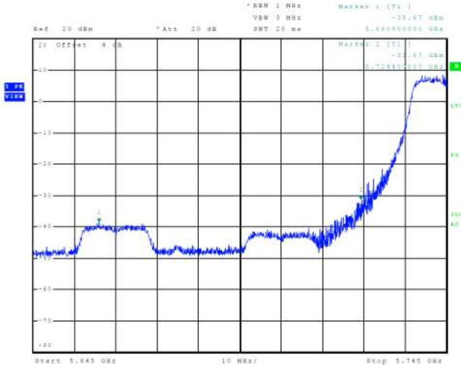
Figure 35 Plot of Transmitter Low Band Edge Chain 1 (5725-5850 MHz Band, 802.11a)
