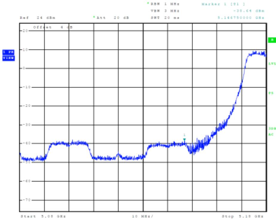
Figure 25 Plot of Transmitter Low Band Edge Chain 1 (5150-5250 MHz Band, 802.11a)
