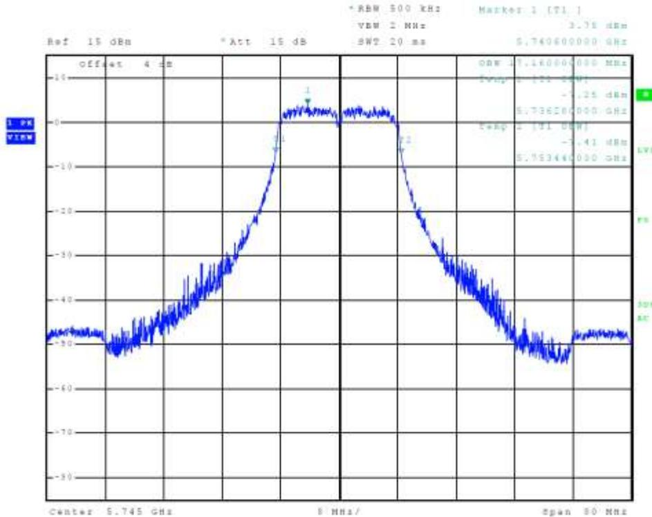
Figure 39 Plot of Transmitter Emissions Chain 1 (5725-5850 MHz Band, 802.11a, 99% OBW)
