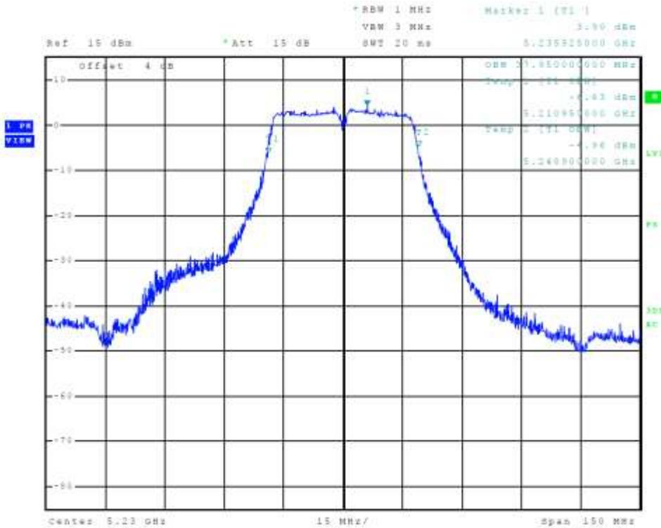
Figure 11 Plot of Transmitter Emissions Chain 0 (5150-5250 MHz Band, 802.11n40, 99% OBW)
