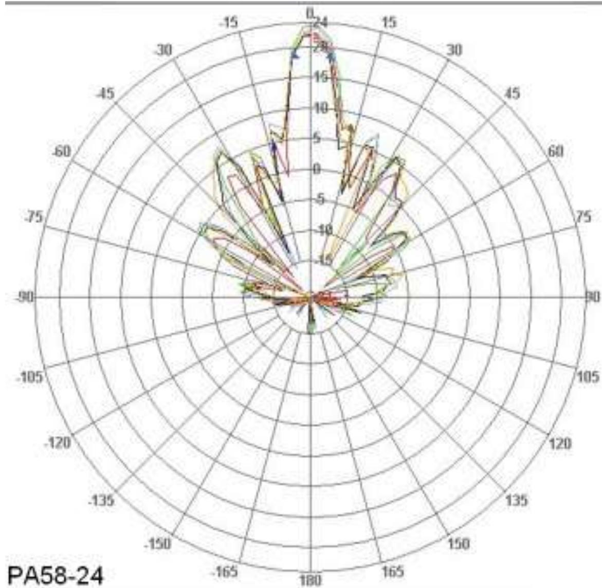
**Elevation Compliance Dish Antenna (32 dBi) HDDA5W-32-DP2**
