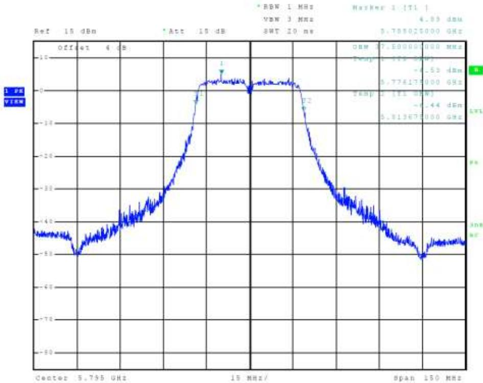
Figure 41 Plot of Transmitter Emissions Chain 1 (5725-5850 MHz Band, 802.11n40, 99% OBW)
