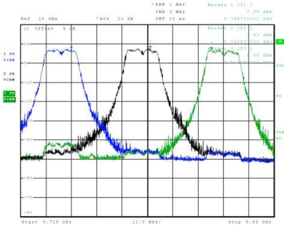
Figure 13 Plot of Transmitter Emissions Chain 0 (Across 5725-5850 MHz Band, 802.11a)
