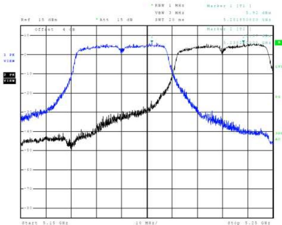
Figure 24 Plot of Transmitter Emissions Chain 1 (Across 5150-5250 MHz Band, 802.11n40)
