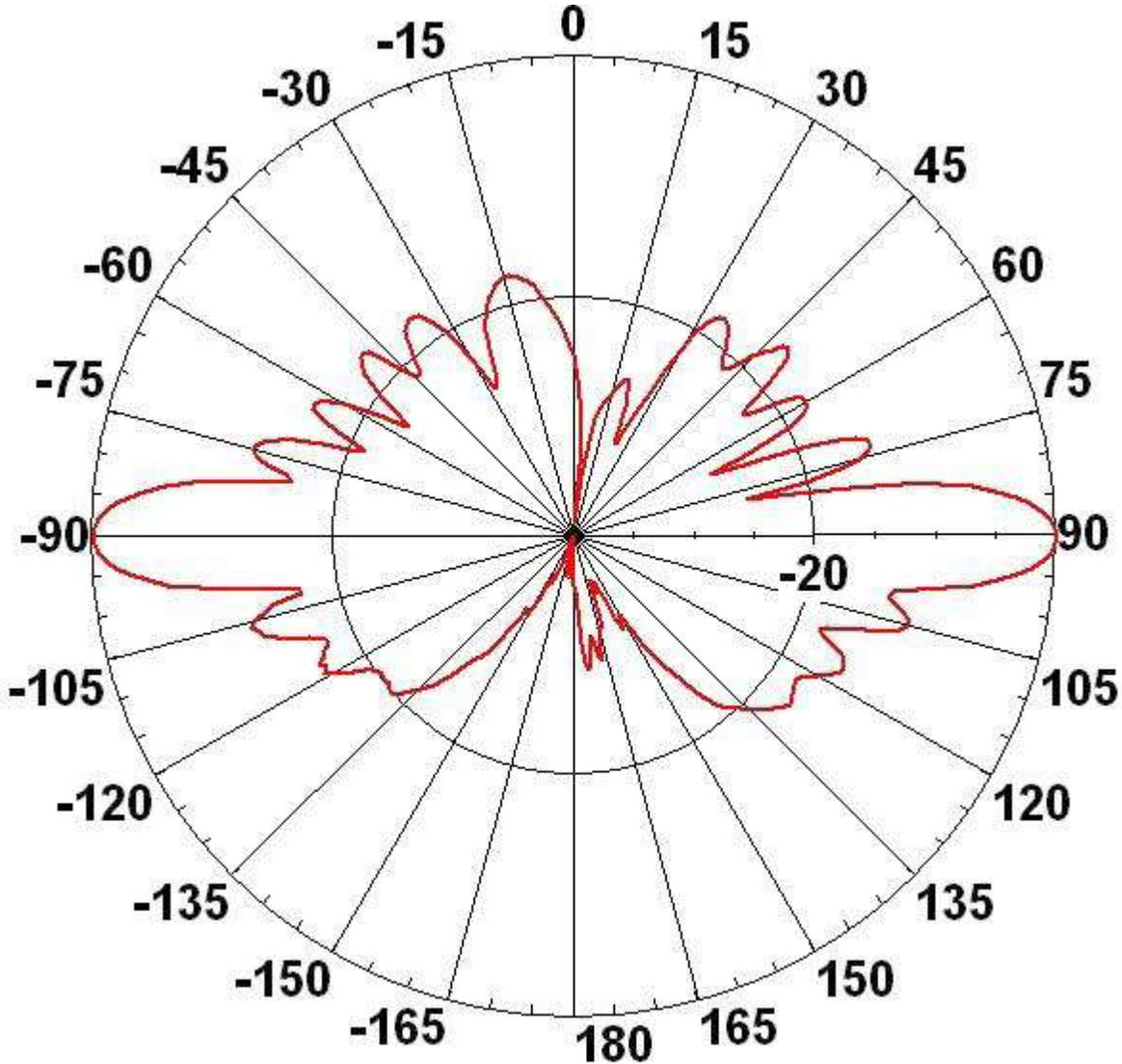
**Elevation Compliance Panel Antenna (24 dBi) PA58-24-ANT**
