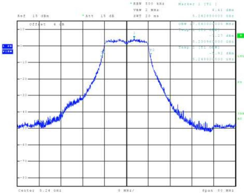
Figure 9 Plot of Transmitter Emissions Chain 0 (5150-5250 MHz Band, 802.11a, 99% OBW)
