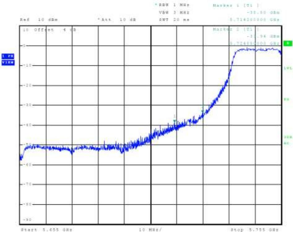
Figure 16 Plot of Transmitter Low Band Edge Chain 0 (5725-5850 MHz Band, 802.11n40)
