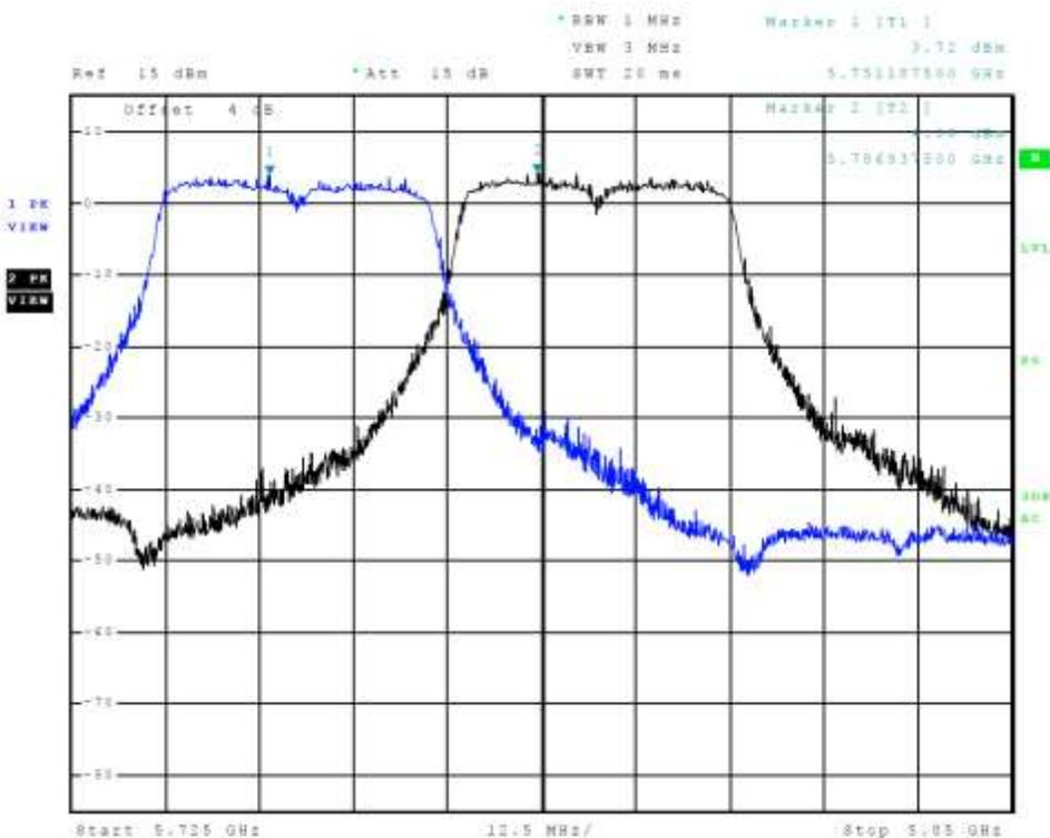
Figure 34 Plot of Transmitter Emissions Chain 1 (Across 5725-5850 MHz Band, 802.11n40)
