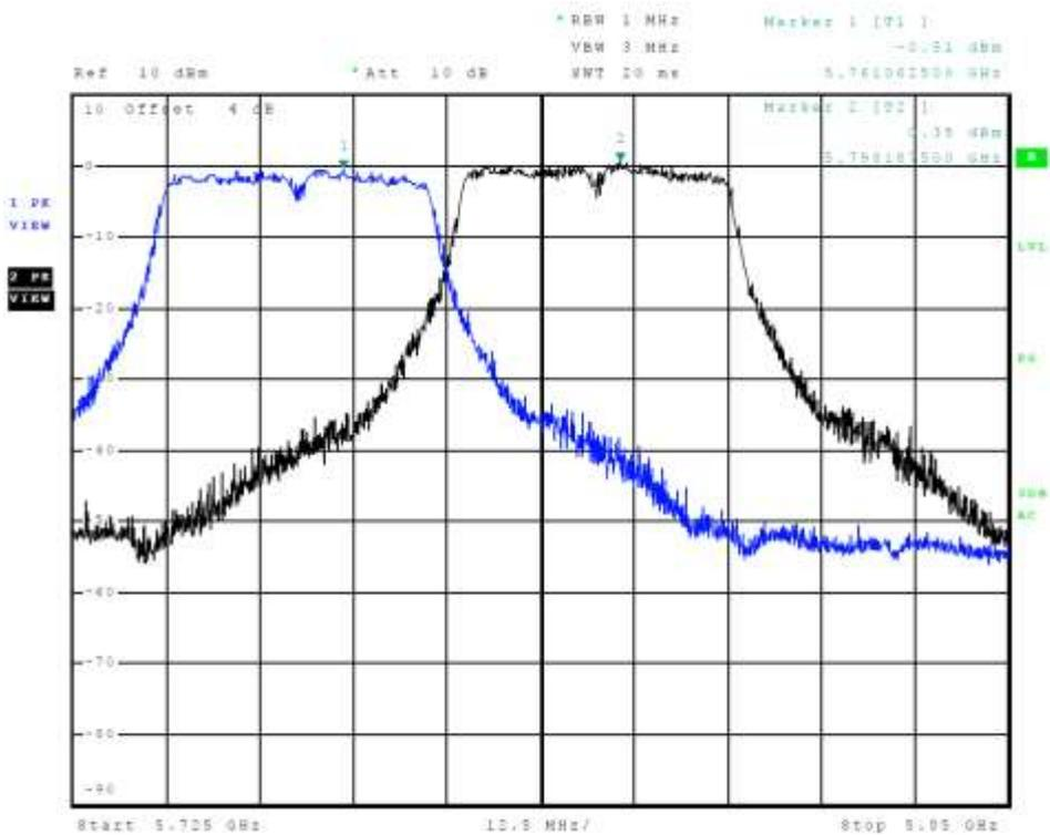
Figure 14 Plot of Transmitter Emissions Chain 0 (Across 5725-5850 MHz Band, 802.11n40)
