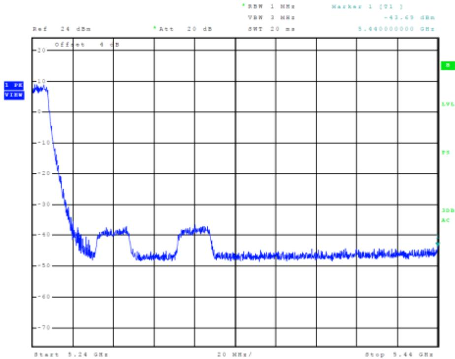
Figure 27 Plot of Transmitter High Band Edge Chain 1 (5150-5250 MHz Band, 802.11a)
