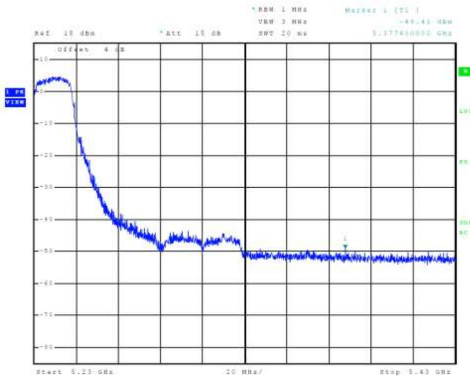
**Figure 8 Plot of Transmitter High Band Edge Chain 0 (5150-5250 MHz Band, 802.11n40)**
