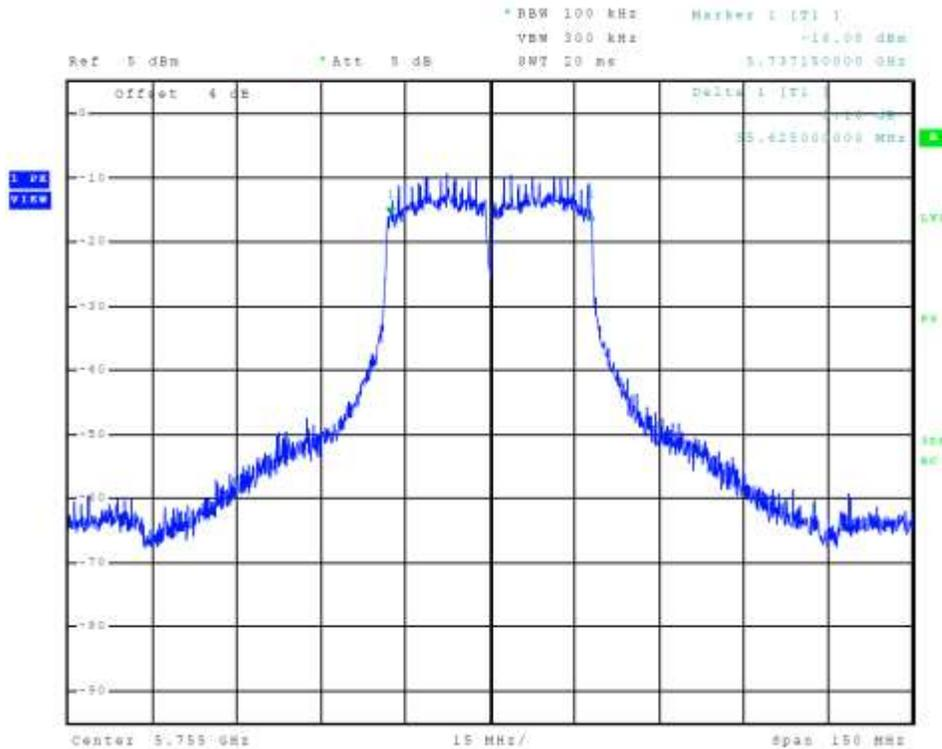
Figure 22 Plot of Transmitter Emissions Chain 0 (5725-5850 MHz Band, 802.11n40, 6-dB OBW)
