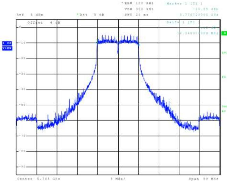
Figure 40 Plot of Transmitter Emissions Chain 1 (5725-5850 MHz Band, 802.11a, 6-dB OBW)
