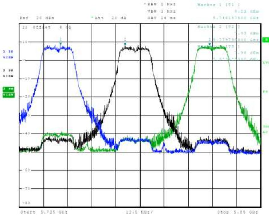
Figure 33 Plot of Transmitter Emissions Chain 1 (Across 5725-5850 MHz Band, 802.11a)
