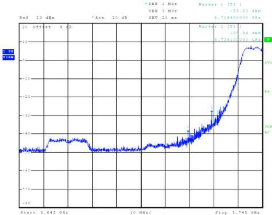
Figure 15 Plot of Transmitter Low Band Edge Chain 0 (5725-5850 MHz Band, 802.11a)
