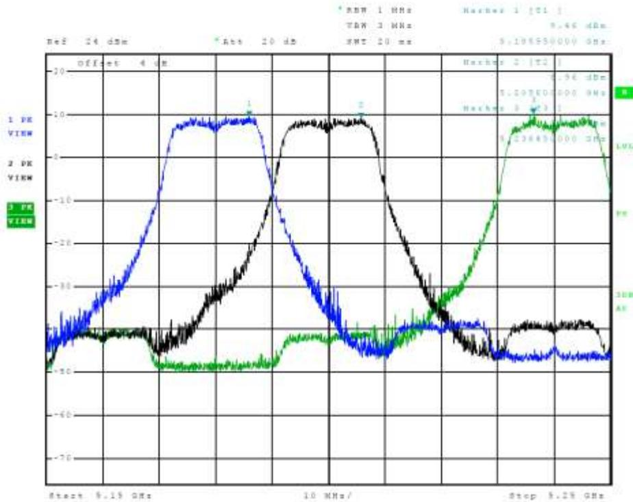
Figure 23 Plot of Transmitter Emissions Chain 1 (Across 5150-5250 MHz Band, 802.11a)
