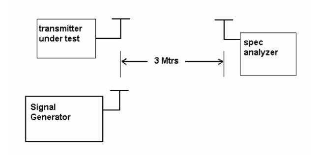
Method of Measurements: The tabulated data shows the results of the radiated field strength emissions test. The spectrum was scanned from 30 MHz to at least the tenth harmonic of the fundamental. This test was conducted per TIA/EIA STANDARD 603 using the substitution method.
