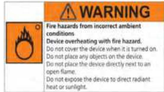
devolo devices should only be installed in locations that guarantee adequate ventilation. Slots and openings on the housing are used for ventilation.
