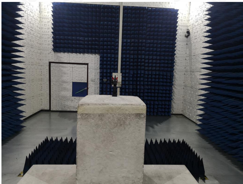
FCC RADIATED EMISSION TEST SETUP ABOVE 1GHZ
