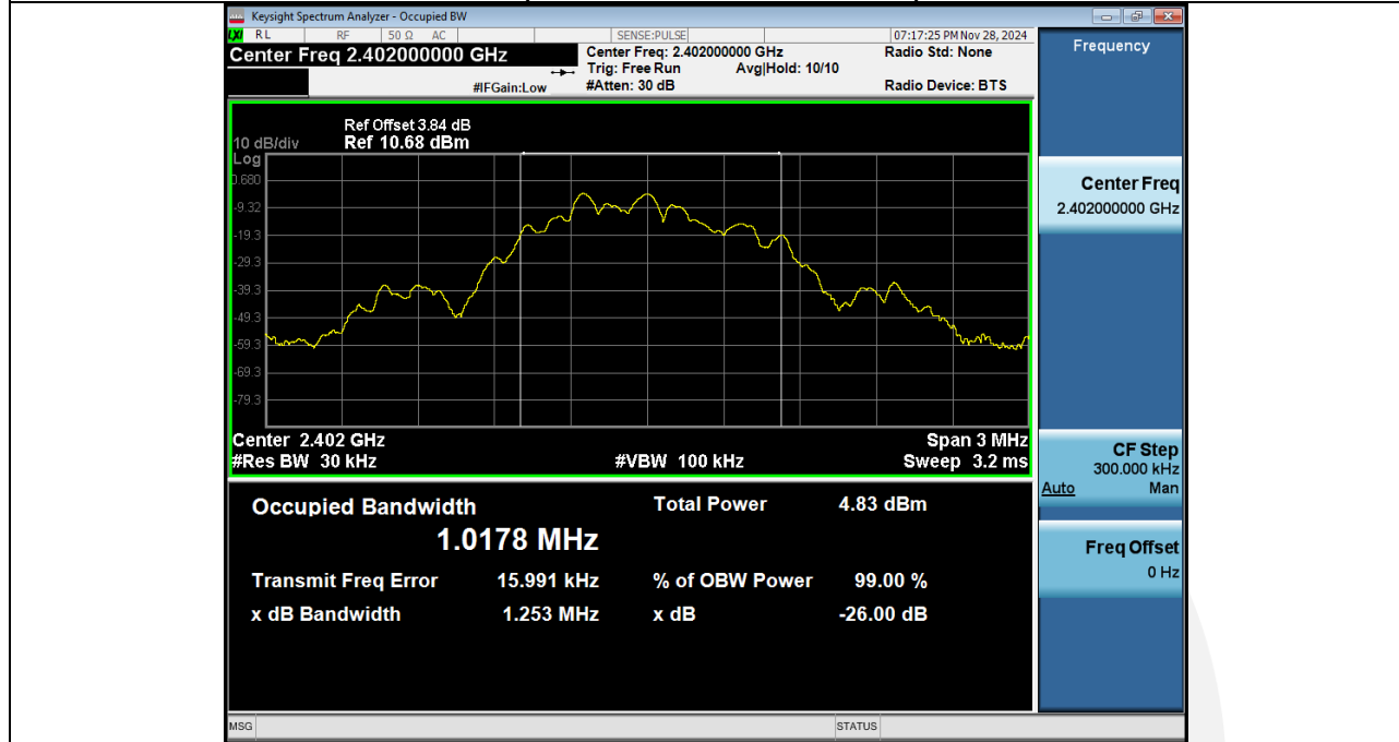
99% Occupied Bandwidth NVNT ANT1 1Mbps 2402
