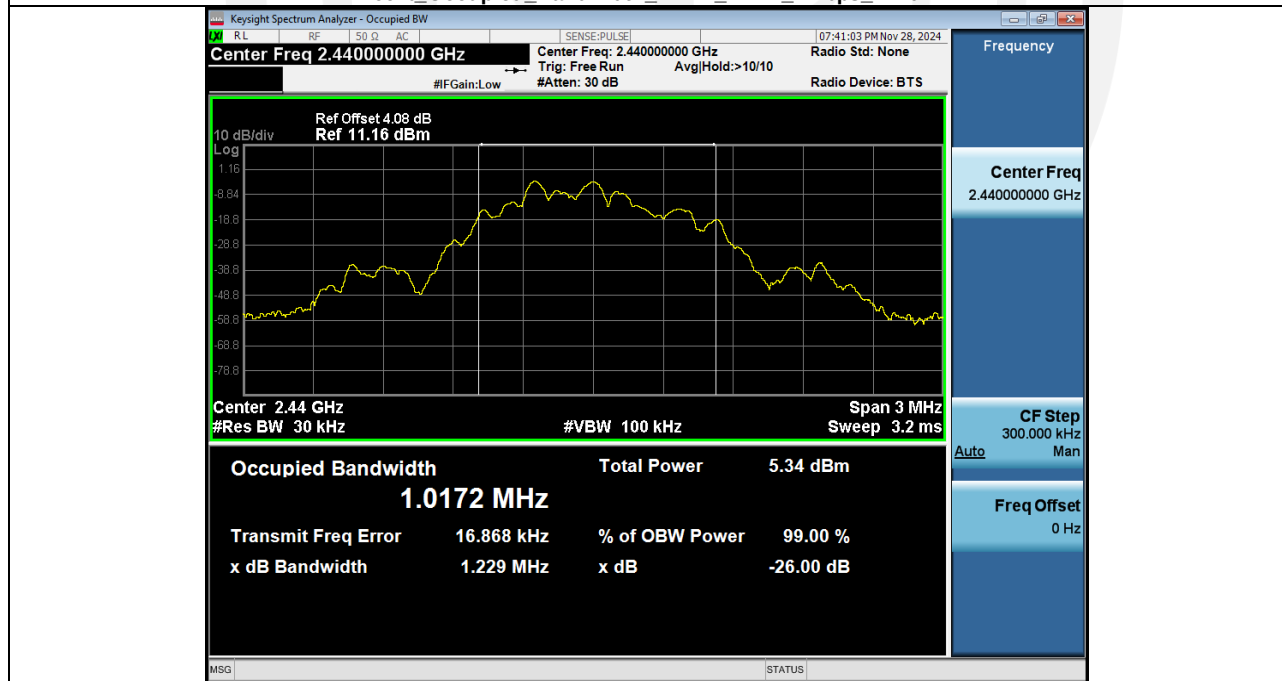
99% Occupied Bandwidth NVNT ANT1 1Mbps 2440
