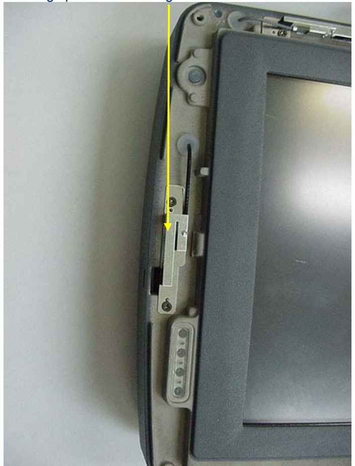
Photograph A.1-6 - Left Edge Bluetooth Antenna Location
