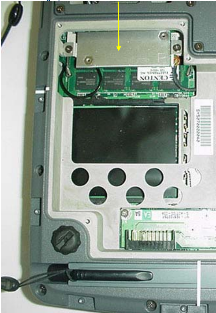
Photograph A.1-5 - Internal Bluetooth Location
