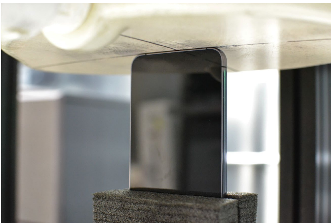
SAR Test Setup Photo 14 – Phablet, Bottom Edge at 0mm
