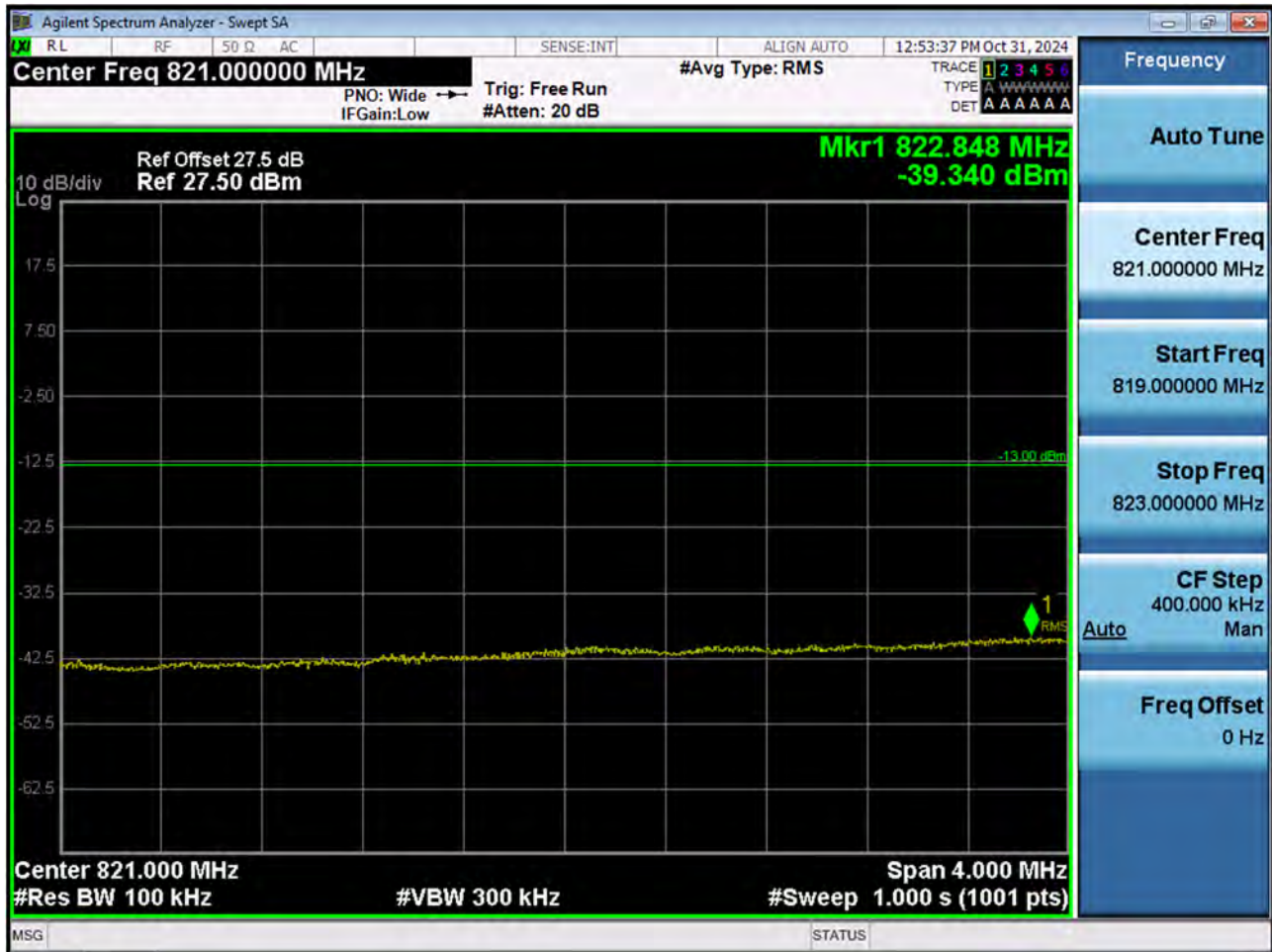
BAND 26. Upper Extended Band Edge Plot (3 M BW Ch.27025 QPSK_RB15_0)
