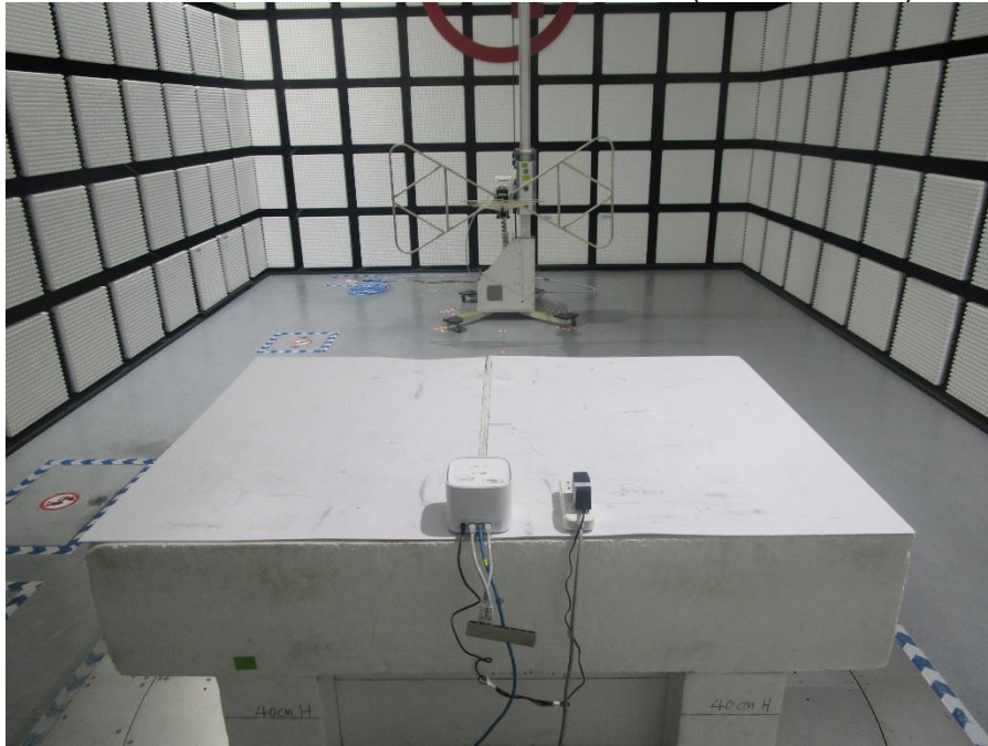
POWERLINE CONDUCTED EMISSIONS MEASUREMENT SETUP
