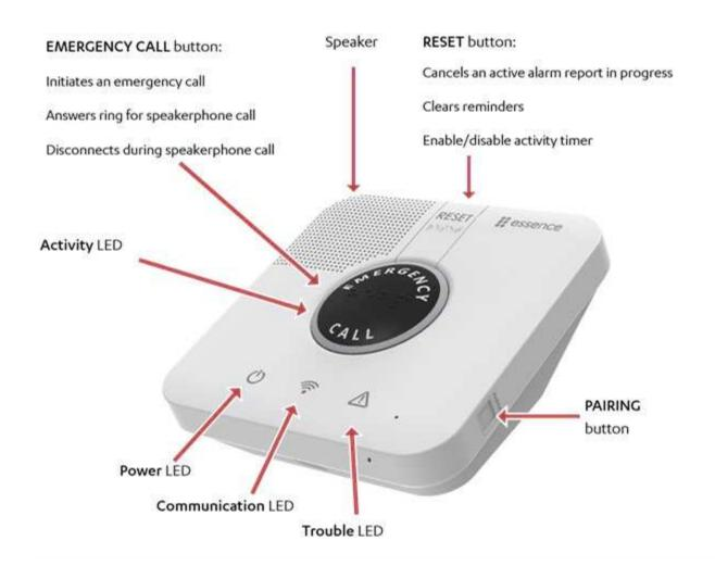
The C7000 includes a high-volume speaker, and a sensitive microphone. The **EMERGENCY CALL** and **RESET** buttons on the C7000, include raised braille characters, for ease of use by visually impaired residents.
