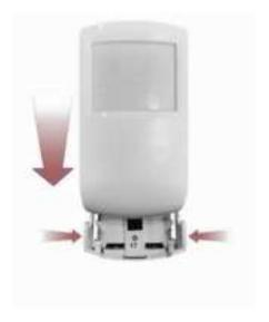
5. Slide the battery compartment upward into the MDsense until it clicks. The LED flashes.
