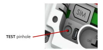
The C7000 LEDs flash and the C7000 beeps three times. The C7000 is restored to factory settings.
