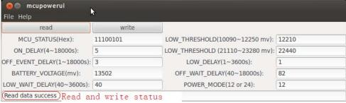
d. Example of the method of changing the low DC input voltage detection value:
