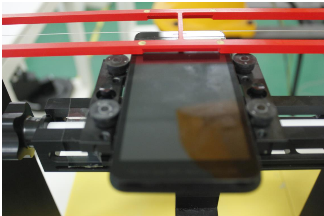
Picture 2: EUT Positioning for RF/T-coil
