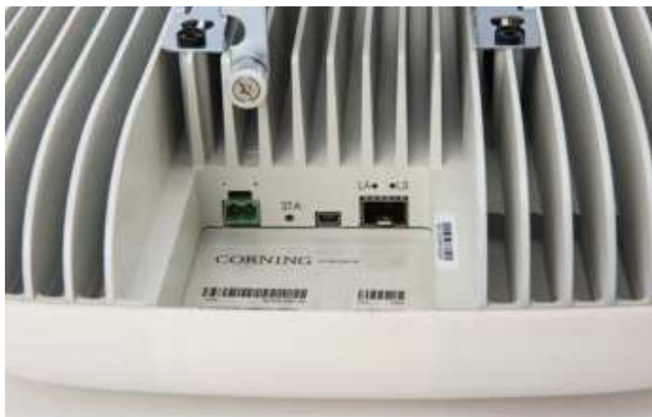
Figure 4 SCRN-520 Connectors and Status LED
