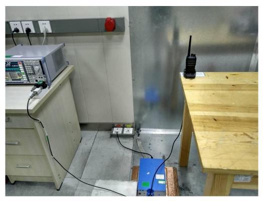
RADIATED EMISSION TEST SETUP
