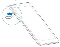
Pull out the card tray and place the nano-SIM card and the optional microSDXC card on the tray, as shown.
