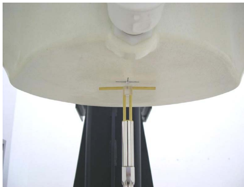
Picture 8.2 Photo of Dipole Setup
