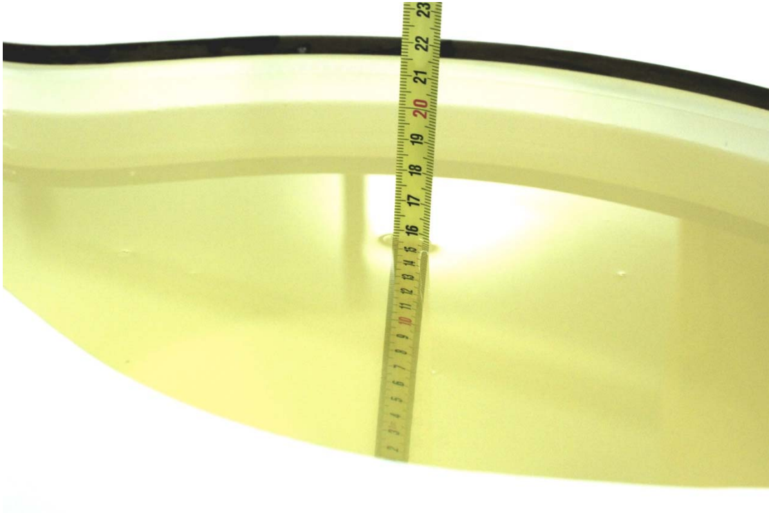
Picture 7-3 Liquid depth in the Flat Phantom (2600MHz)
