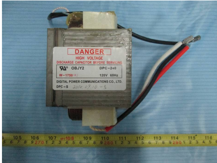
EUT – Power Transformer View
