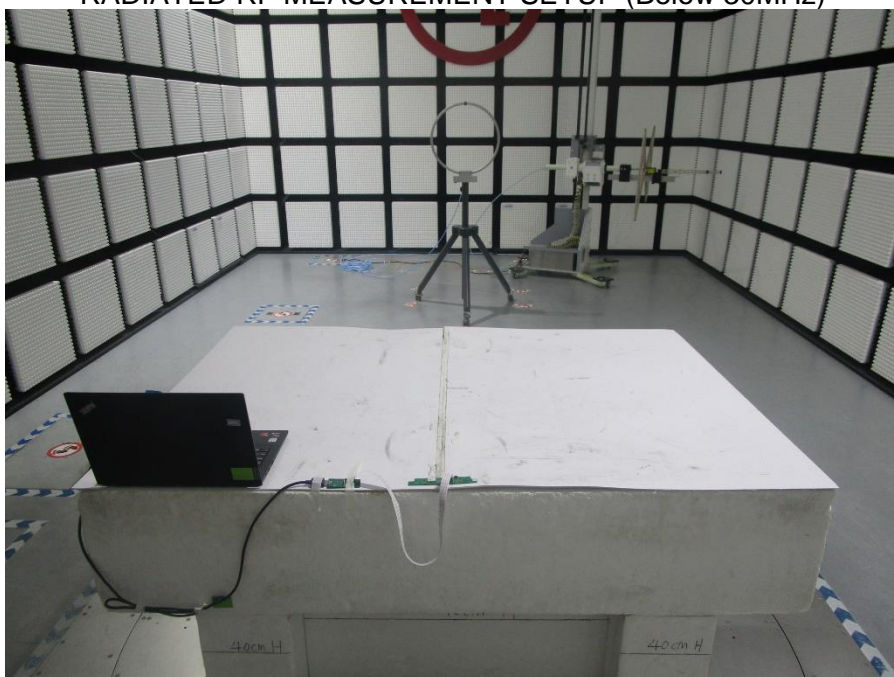
RADIATED RF MEASUREMENT SETUP (Below 30MHz)
