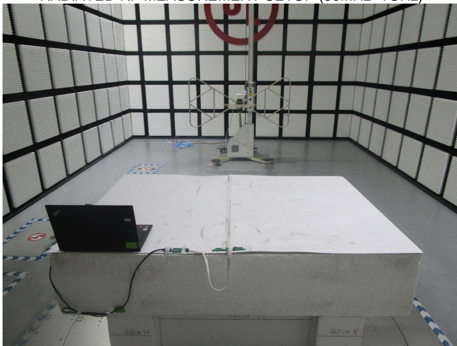
RADIATED RF MEASUREMENT SETUP (Below 30MHz)
