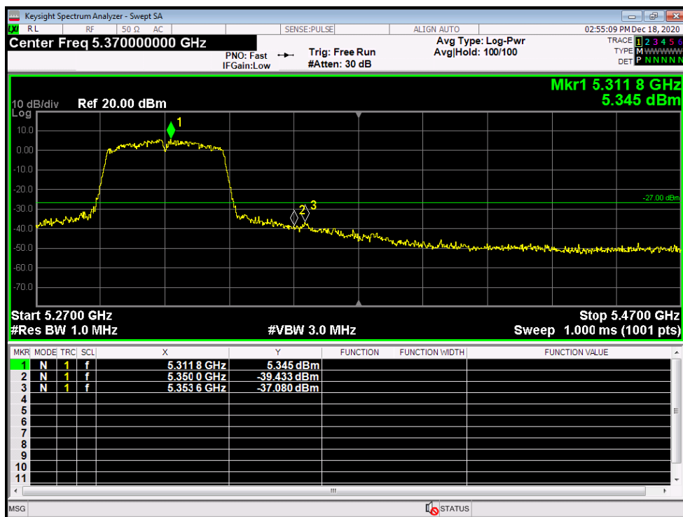
Band Edge NVNT ac80 5290MHz Low Ant1
