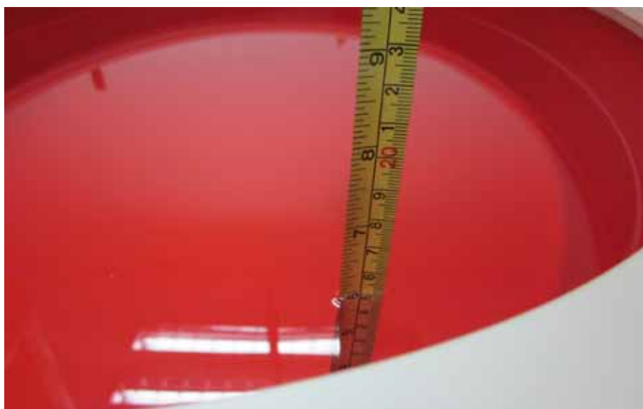
Figure 4.4: Liquid depth in the Flat Phantom
