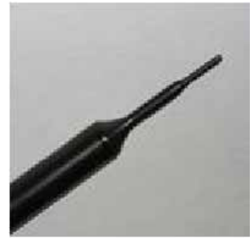
Figure 4.4 EX3DV4 E-field Probe
