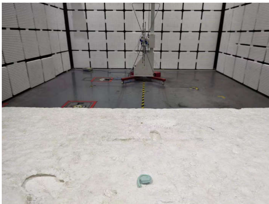
Radiated spurious emission Test Setup-3(Below 1GHz)(right ear)
