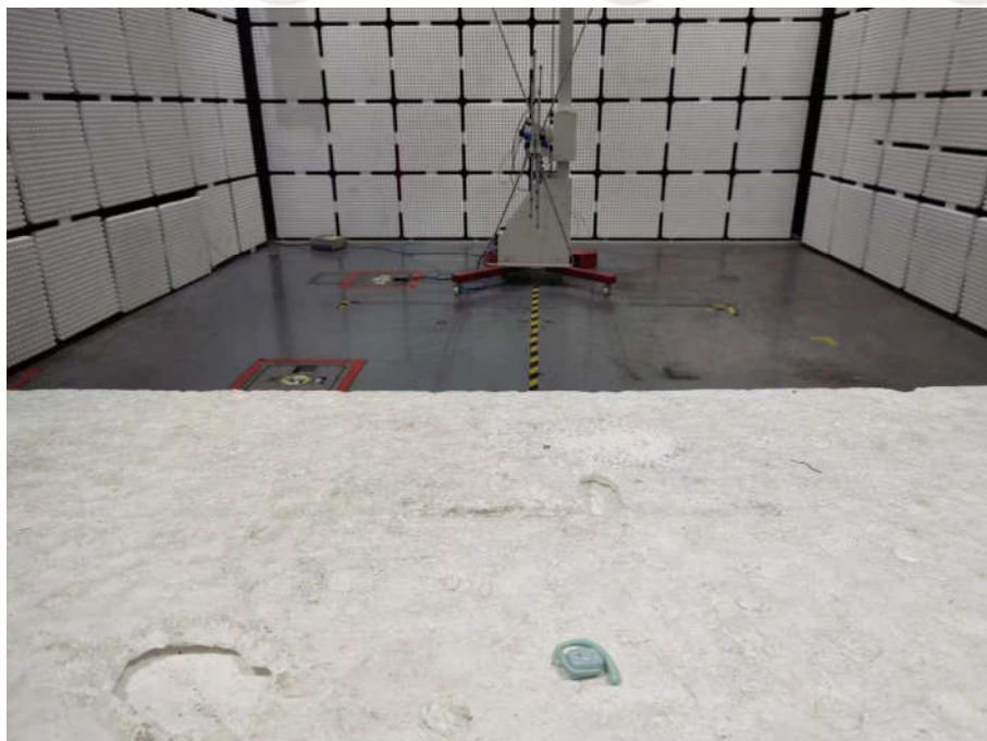
Radiated spurious emission Test Setup-1(Below 1GHz)(left ear)
