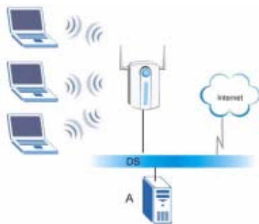
Figure 9 WPA with RADIUS Application Example
