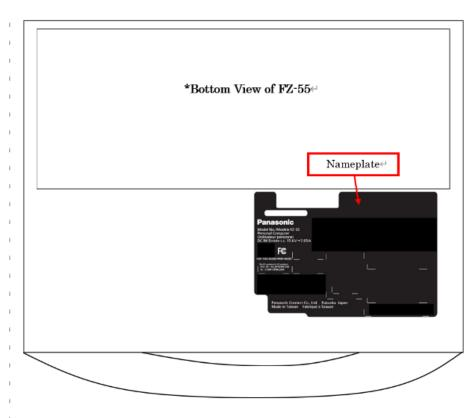
The name plate is to be affixed to the host PC FZ-55 using strong adhesive on its backside.
