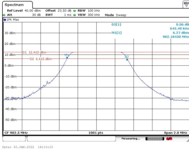
6 dB Bandwidth Plot on Channel 31
