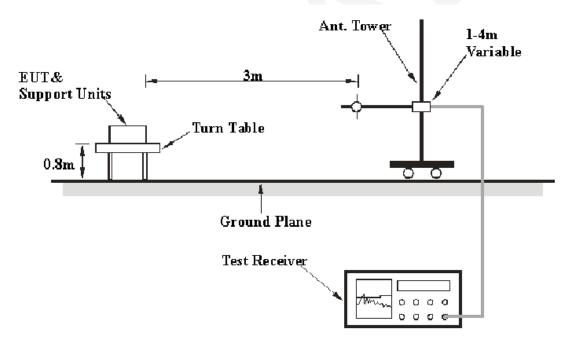
The radiated emission tests were performed in the 3 meters test site, using the setup accordance with the ANSI C63.17 - 2006. The specification used was the FCC 15§ 15.319(g).
