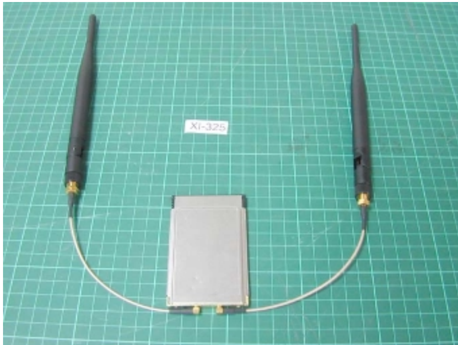
Photo 2: EUT with antenna (antenna gain is 5dBi)
