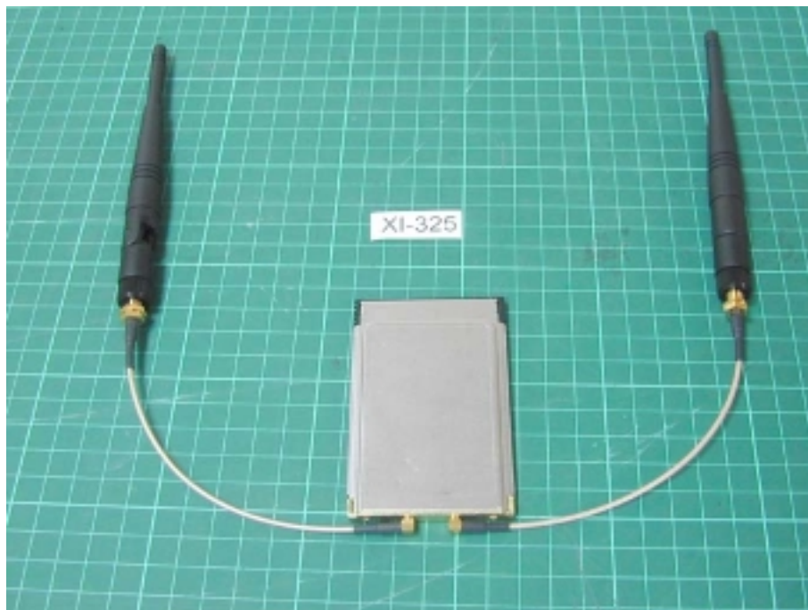
Photo 3: EUT with antenna (antenna gain is 2dBi)
