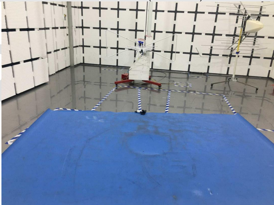
Radiated Emissions (30MHz-1GHz)
