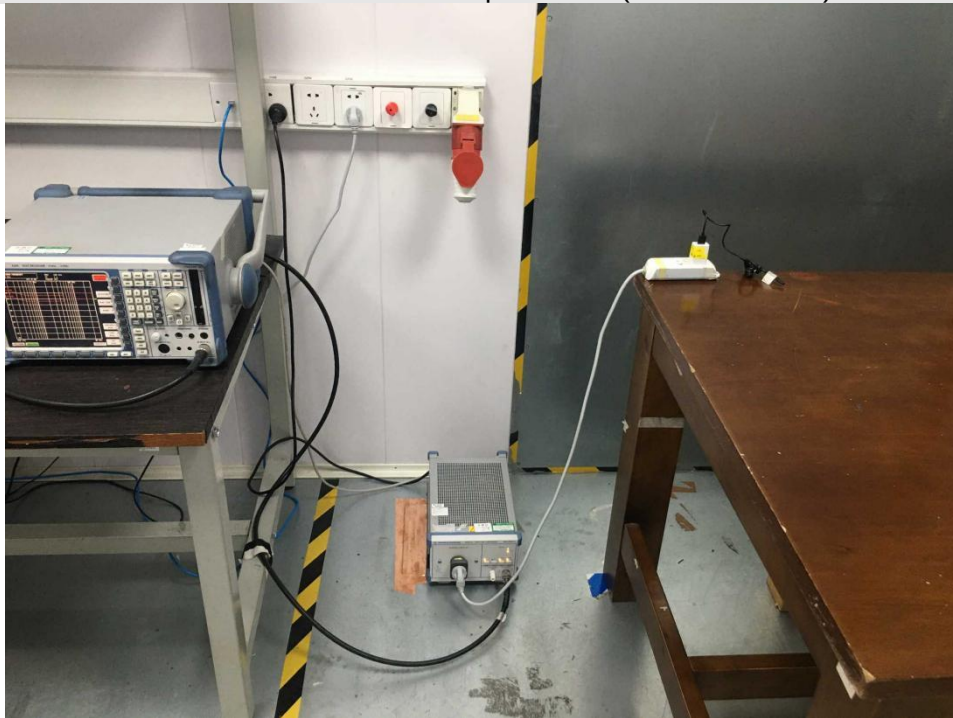
Conducted emissions at AC power line (150kHz-30MHz)
