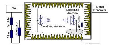
In the chamber, a substitution antenna for the frequency band of interest is placed at the reference point of the chamber. An RF Signal source for the frequency band of interest is connected to the substitution antenna with a cable that has been constructed to not interfere with the radiation pattern of the antenna. A power (P<sub>Mea</sub>) is applied to the input of the
