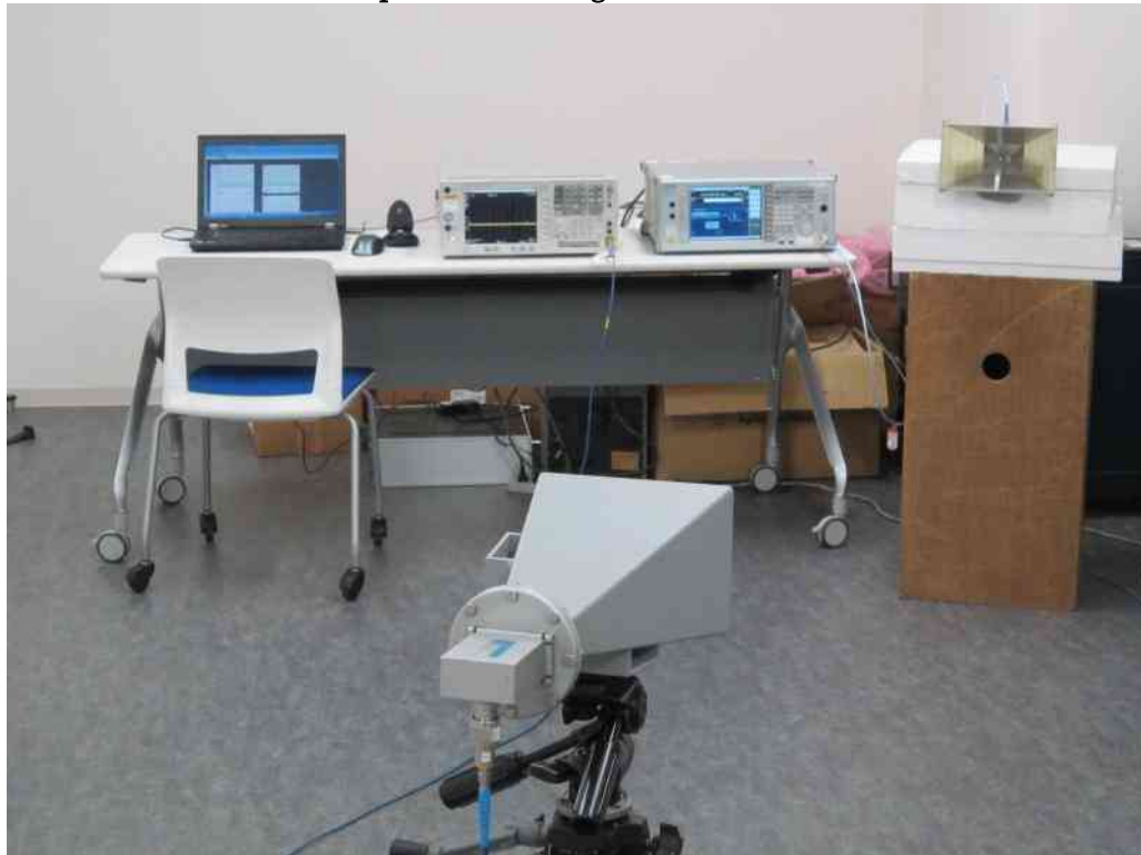
Test Setup for Generating the Radar Waveform
