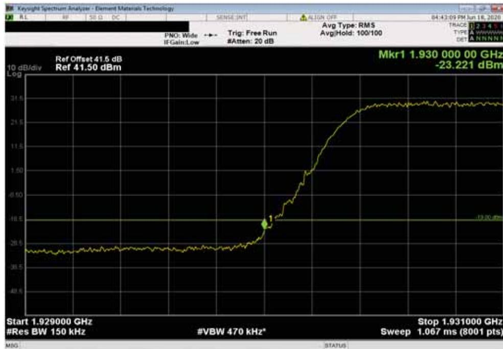
Port 4, Band n25, 1930 MHz - 1995 MHz , 15 MHz Bandwidth, 256-QAM Modulation, Low Channel 1937.5 MHz
