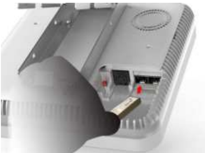
Figure 73. SFP Module Insertion
