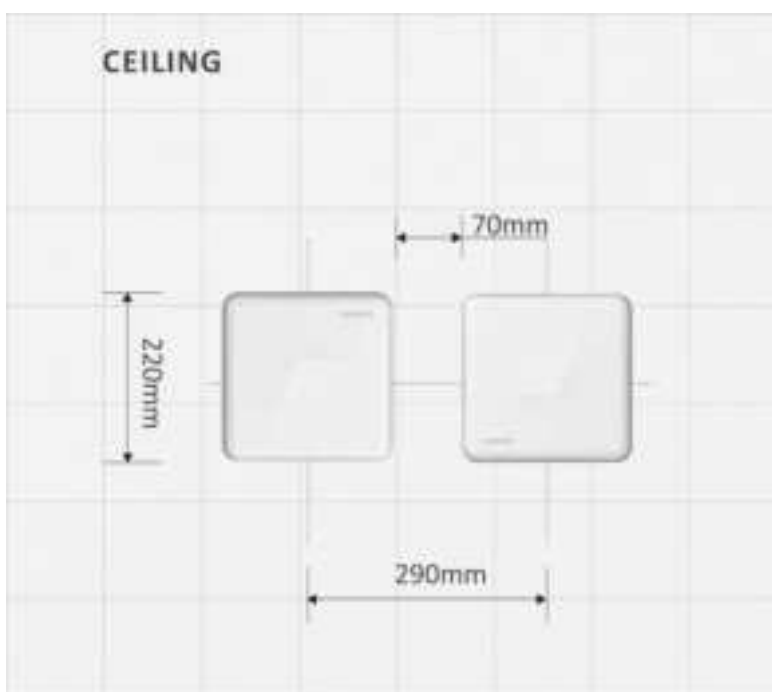
Figure 83. Dual E62-N2RU Clearance
