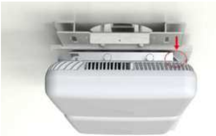
Figure 78. Unlock Rotary Hook Diagram 1
