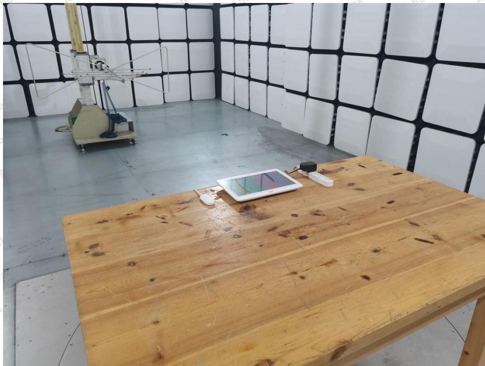
Photo of Radiation Emission Test
