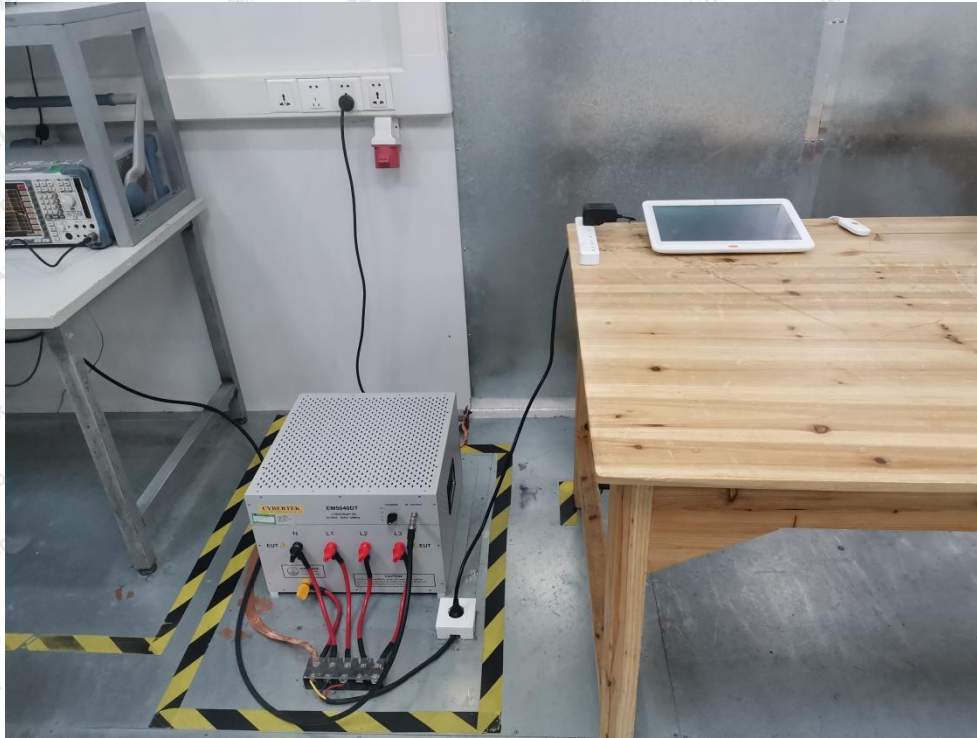
Photo of Conducted Emission Measurement
