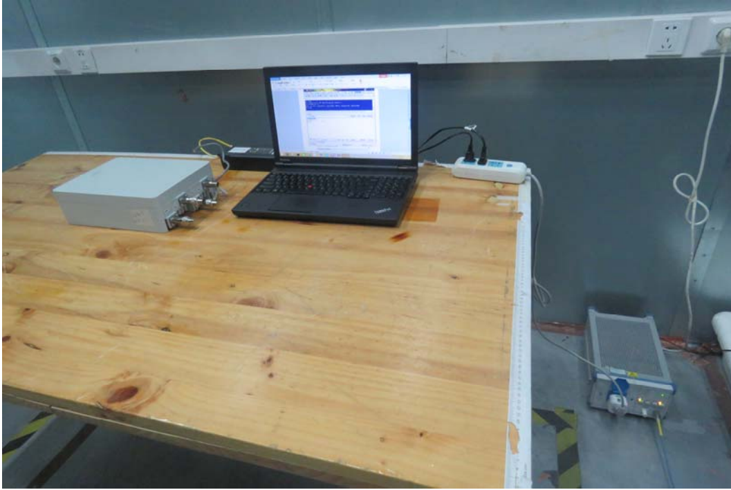
Picture 3 Conducted Emission Test Setup
