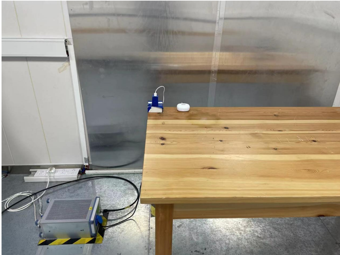
Conducted emission test setup
