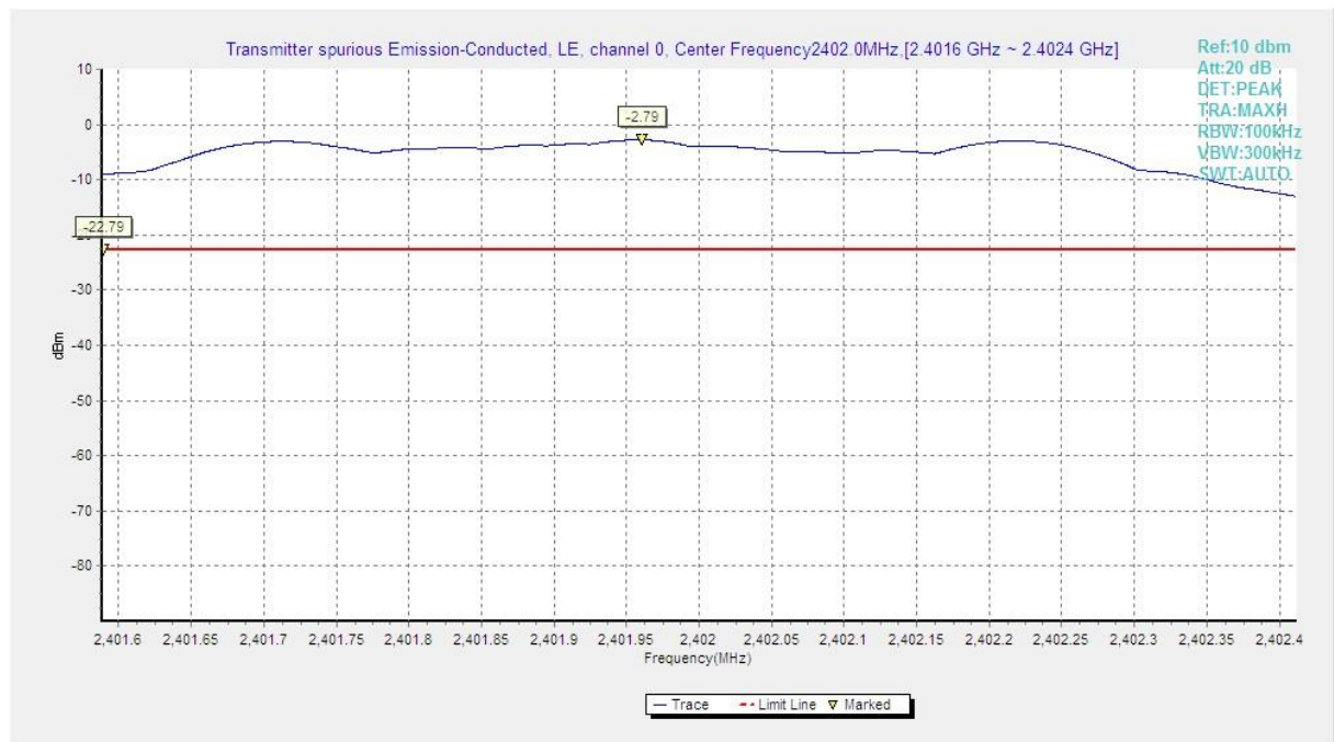
Fig.9 Conducted Spurious Emission (Ch0, Center Frequency)
