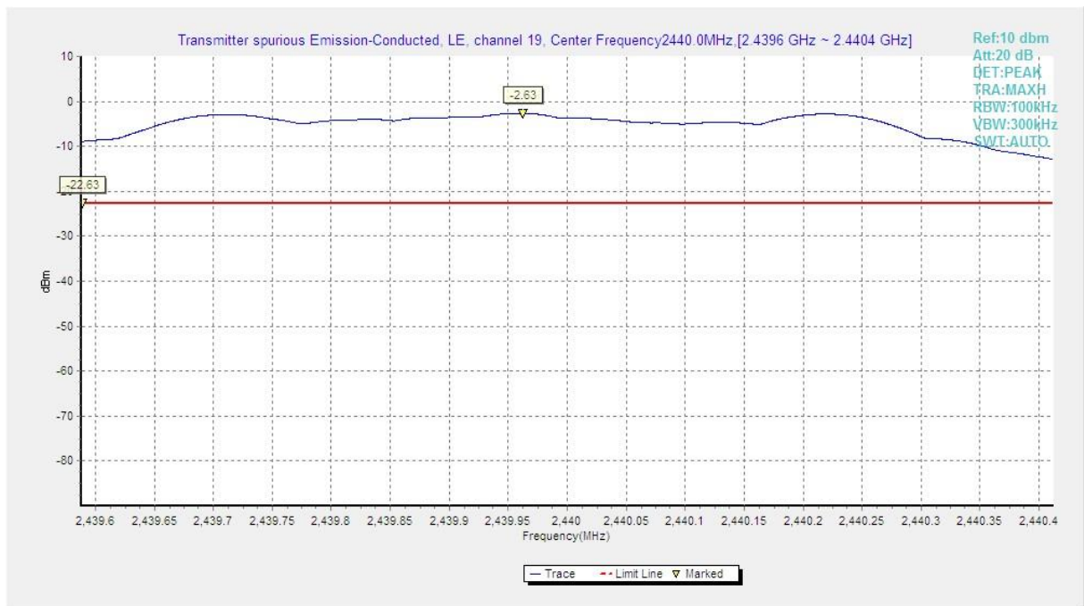
Fig.12 Conducted Spurious Emission (Ch19, Center Frequency)
