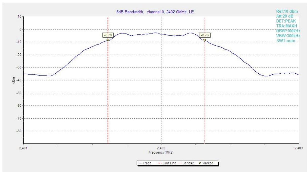
Fig.4 6dB Bandwidth (Ch 0)
