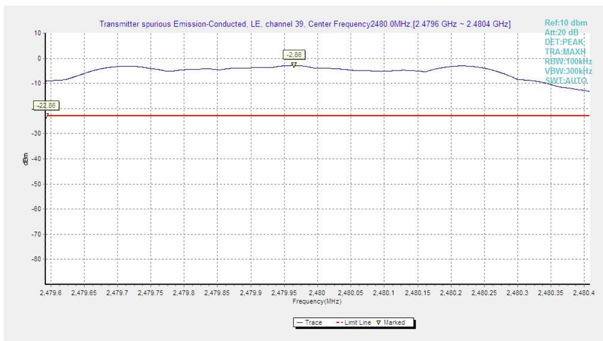
Fig.15 Conducted Spurious Emission (Ch39, Center Frequency)
