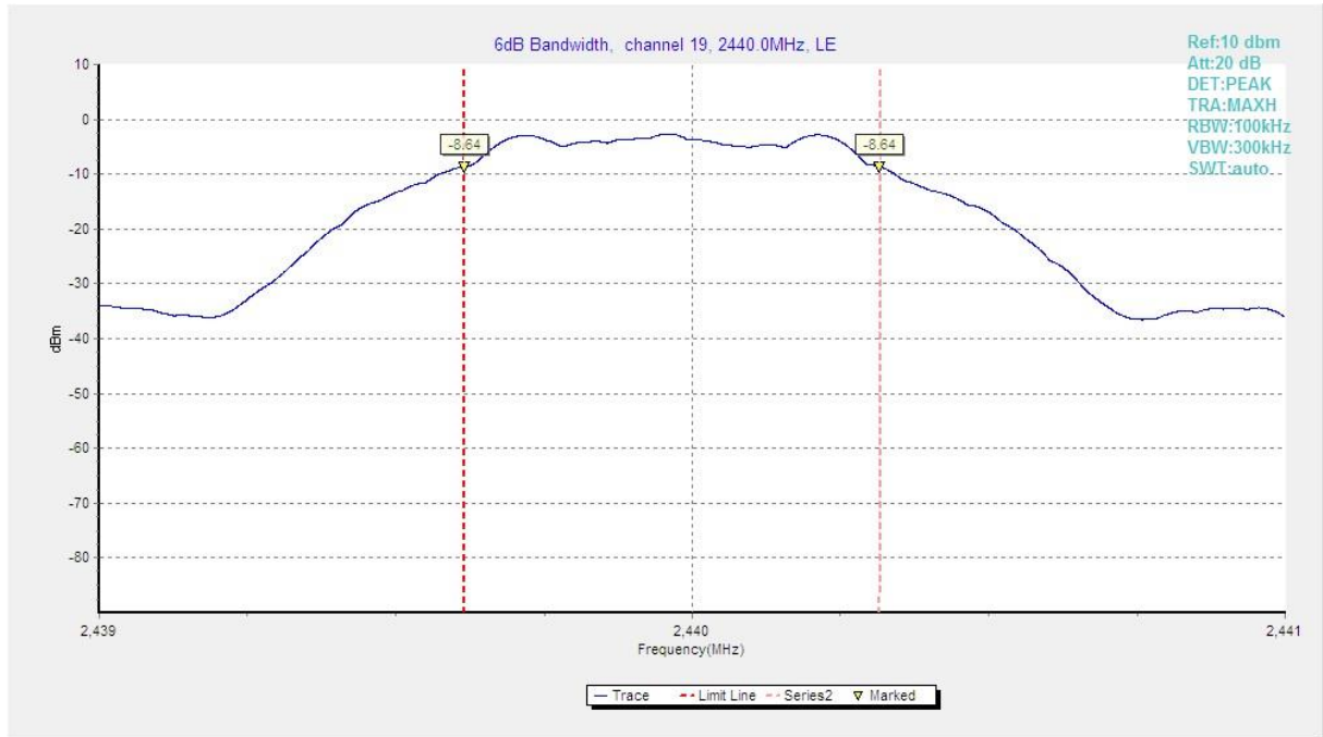
Fig.5 6dB Bandwidth (Ch 19)
