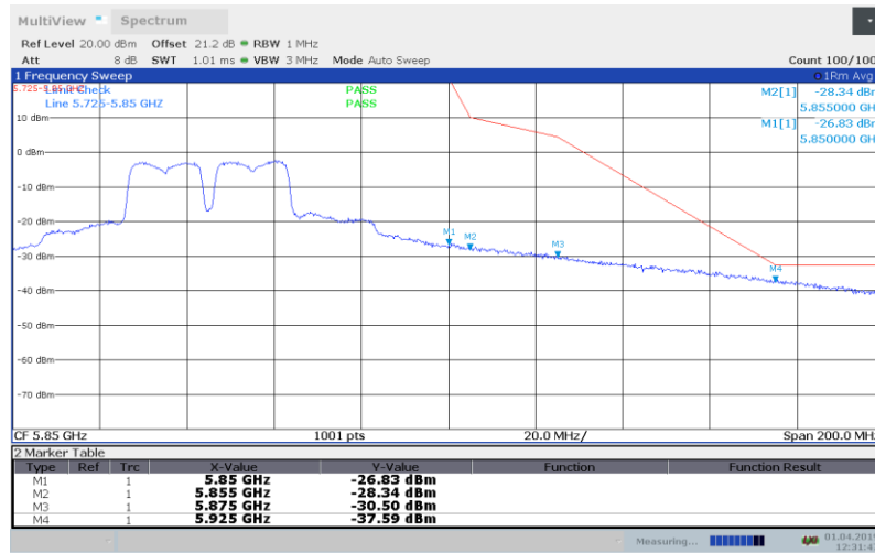
Figure 8.9-24: Conducted emissions at upper band edge measurement, 802.11n
