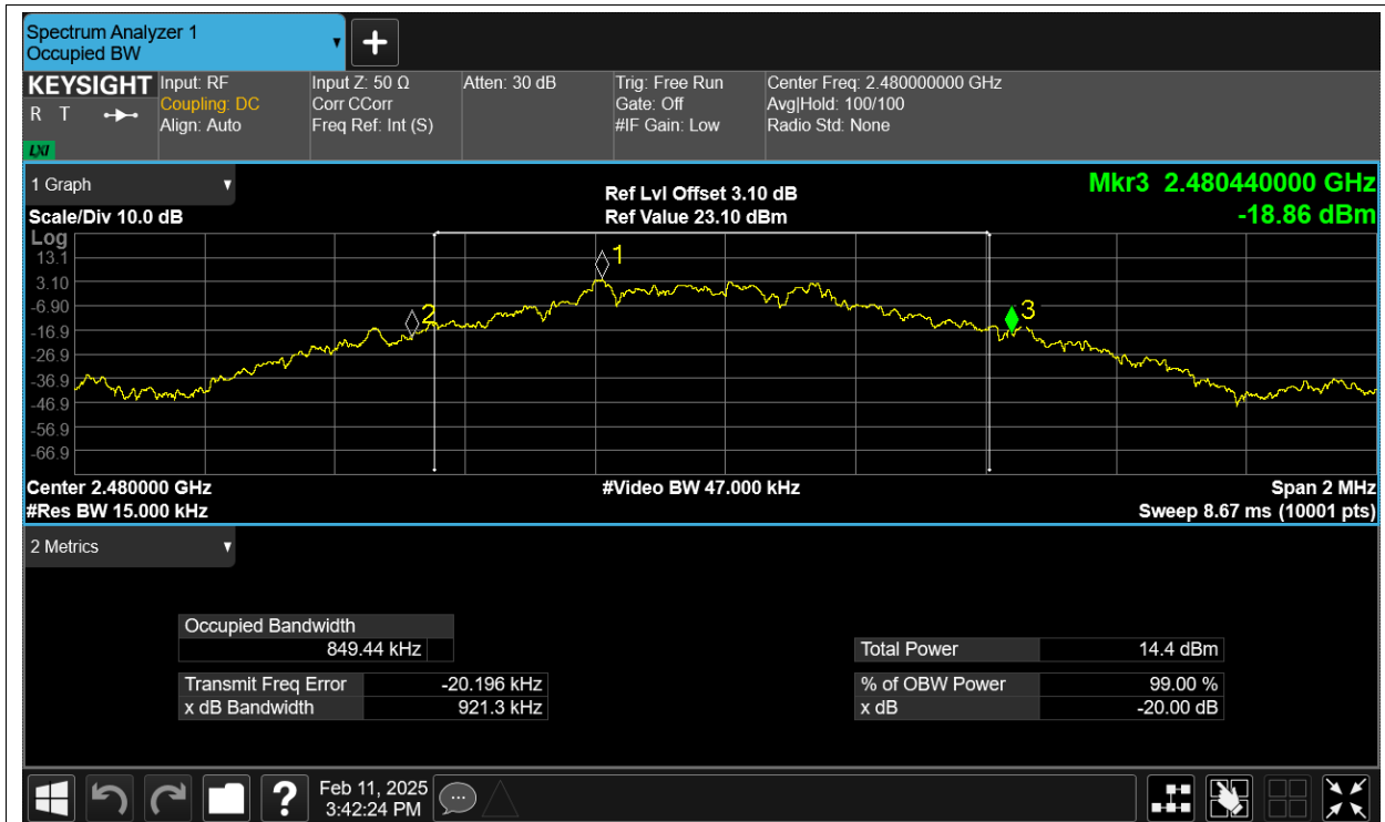
-20dB Bandwidth NVNT 2-DH1 2402MHz Ant1
