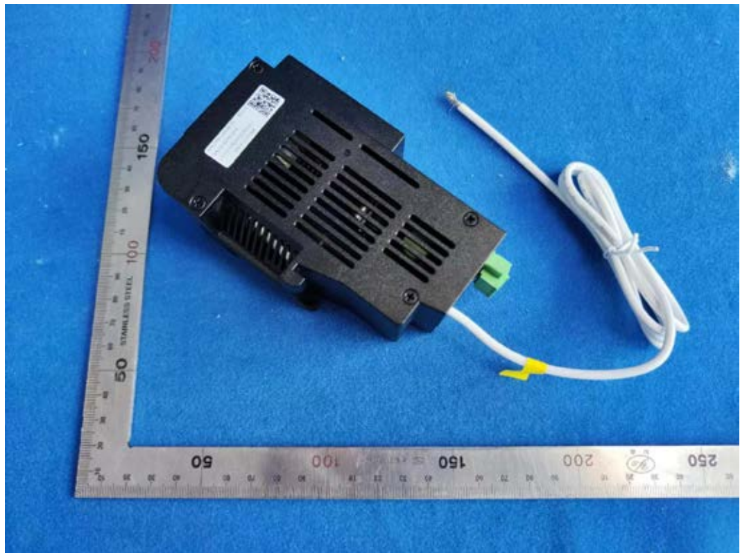
FIGURE 2 1-INCH 2-CHANNEL POWER MONITOR MODULE, PIGTAIL (M/N: GPM-H2SEM-00) GENERAL APPEARANCE TOP VIEW
