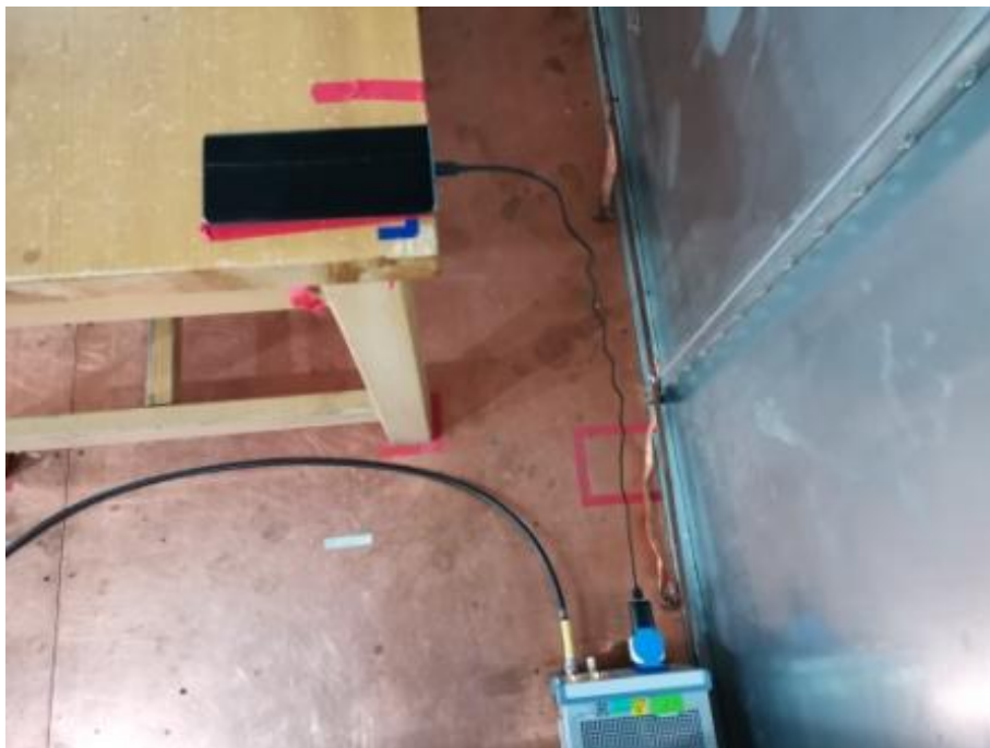
Conducted Emissions Test Setup (with charger)
